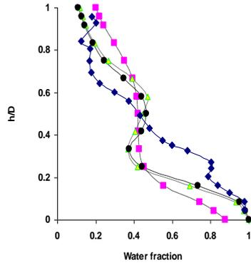
Fig. 2.  $h/D$  versus water fraction with 46% of water in inlet (velocity of mixture is 1.25 m/s):  $\blacklozenge$ - Experimental;  $\blacksquare$ -CFD with PBE (Luo);  $\blacktriangle$ - CFD with PBE (Coulaloglou);  $\bullet$ - CFD with PBE (modified Coulaloglou).
