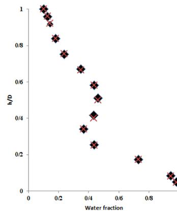
**Fig. 9.**  $h/D$  versus water fraction with 46% of water in inlet (velocity of mixture is 1.25 m/s), (CFD with PBE (modified Coulaloglou)); ♦ 452330 node; × 947282 node.
