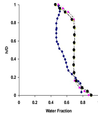
Fig. 5.  $h/D$  versus water fraction with 60% of water in inlet (velocity of mixture is 2.12 m/s):  $\blacklozenge$ - Experimental;  $\blacksquare$ -CFD with PBE (Luo);  $\blacktriangle$ - CFD with PBE (Coulaloglou);  $\bullet$ - CFD with PBE (modified Coulaloglou).
