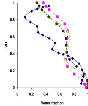
Fig. 4.  $h/D$  versus water fraction with 60% of water in inlet (velocity of mixture is 1.25 m/s):  $\blacklozenge$ - Experimental;  $\blacksquare$ -CFD with PBE (Luo);  $\blacktriangle$ - CFD with PBE (Coulaloglou);  $\bullet$ - CFD with PBE (modified Coulaloglou).
