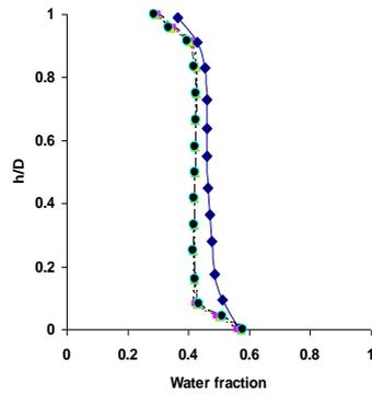
**Fig. 6.**  $h/D$  versus water fraction with 46% of water in inlet (velocity of mixture is 3 m/s): ♦- Experimental; ■-CFD with PBE (Luo); ▲- CFD with PBE (Coulaloglou); ●- CFD with PBE (modified Coulaloglou).
