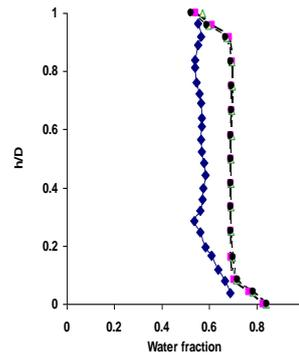
**Fig. 8.**  $h/D$  versus water fraction with 60% of water in inlet (velocity of mixture is 3 m/s): ♦- Experimental; ■-CFD with PBE (Luo); ▲- CFD with PBE (Coulaloglou); ●- CFD with PBE (modified Coulaloglou).
