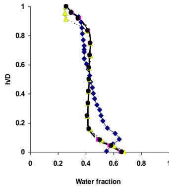
Fig. 3.  $h/D$  versus water fraction with 46% of water in inlet (velocity of mixture is 2.12 m/s):  $\blacklozenge$ - Experimental;  $\blacksquare$ -CFD with PBE (Luo);  $\blacktriangle$ - CFD with PBE (Coulaloglou);  $\bullet$ - CFD with PBE (modified Coulaloglou).
