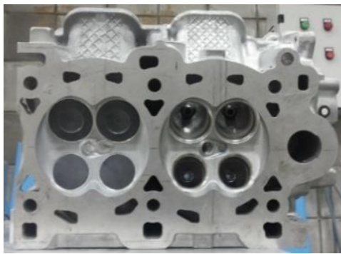
Fig. 2. Spray-guided GDI cylinder head.
