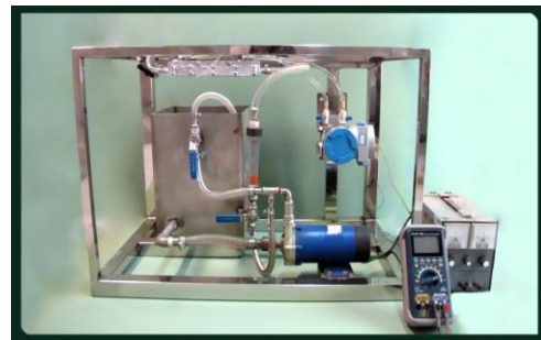
Fig. 9. Experimental setup for measuring pressure drop across the closed channel flow.
