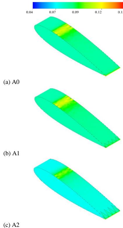
**Fig. 12. RMS pressure fluctuations on airfoil surface.**
