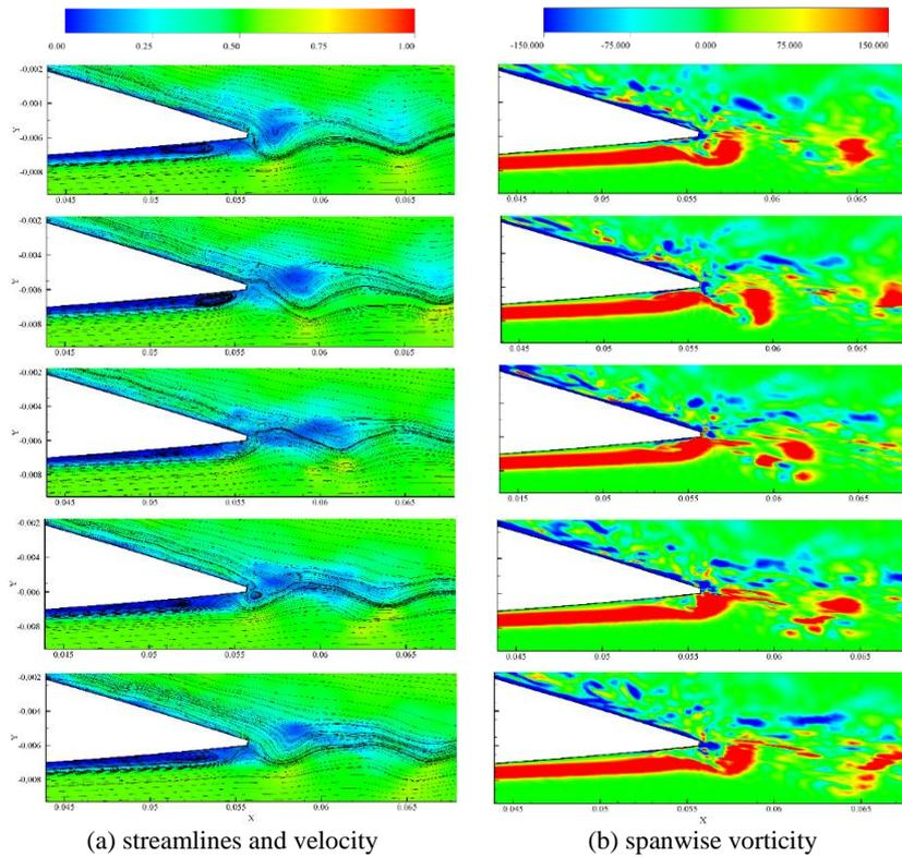
**Fig. 20. Instantaneous flows near trailing edge of A2 (on  $Z_m$ ), top to down:  $t_0$ ~ $t_4$ .**
