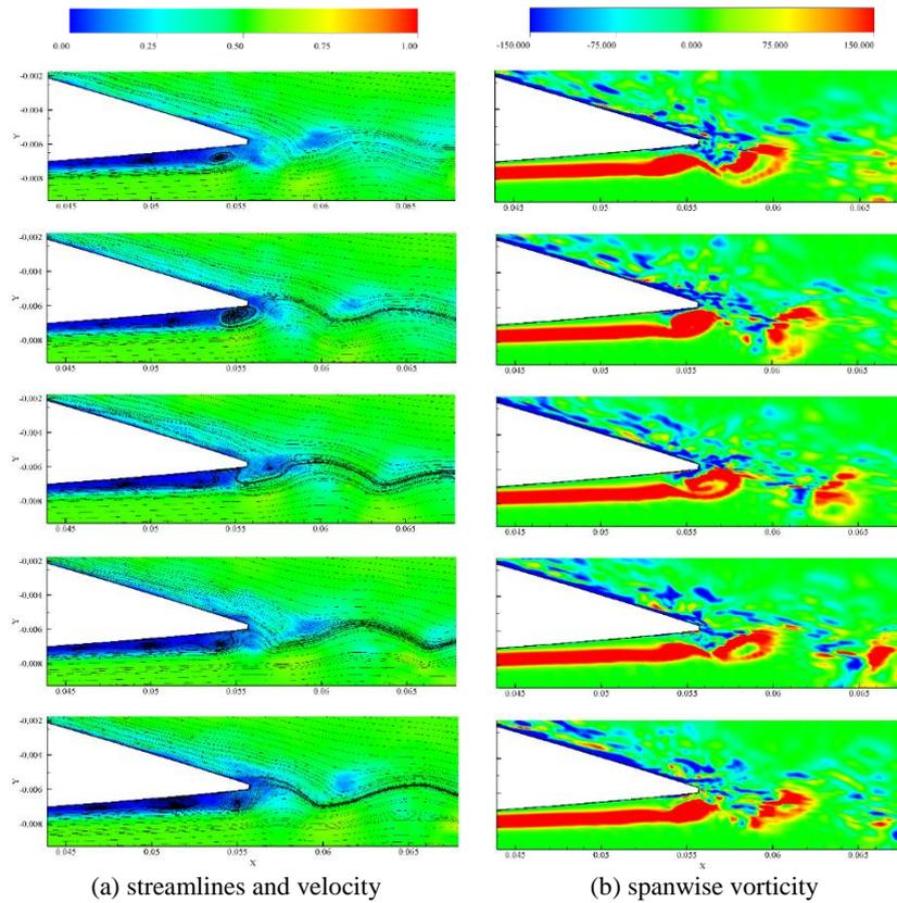
Fig. 18. Instantaneous flows near trailing edge of A1 (on  $Z_m$ ), top to down:  $t_0$ ~ $t_4$ .
