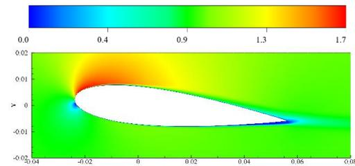
Fig. 7. Time-averaged velocity amplitude of case A0 (on  $Z_m$ ).
