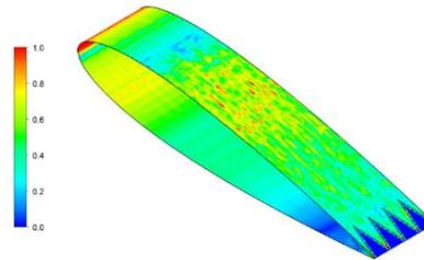
**Fig. 5. Instantaneous  $y^+$  distribution on A2 surface.**
