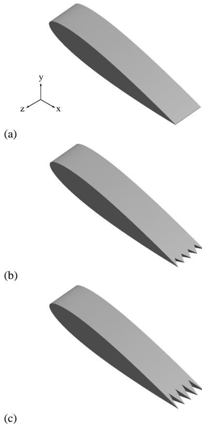
Fig. 2. Airfoil geometry (a) baseline A0, (b) and (c) airfoil with serrated trailing edges A1 and A2.
