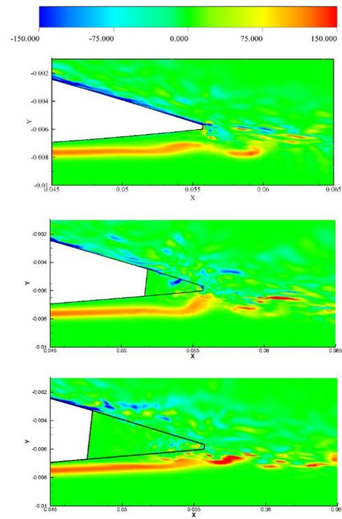
**Fig. 25.** Spanwise vorticity near saw tooth ( $Z_r$ ), top to bottom: A0, A1, A2.
