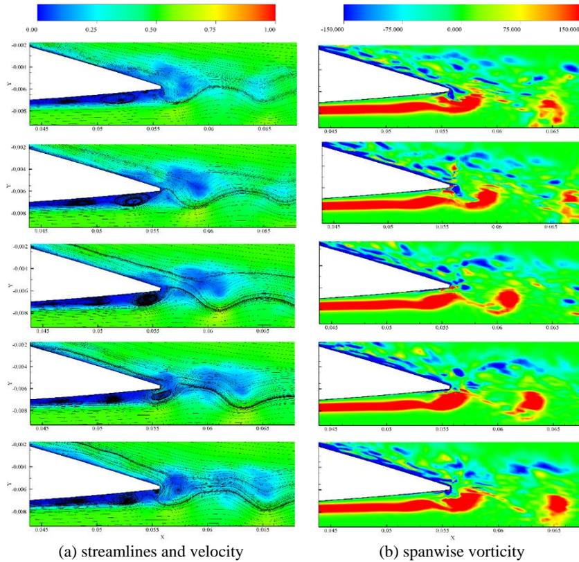
**Fig. 16. Instantaneous flows near trailing edge of A0 (on  $Z_m$ ), top to down:  $t_0$ ~ $t_4$ .**
