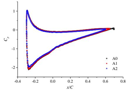
**Fig. 11. Pressure coefficients of airfoils (on Zr).**
