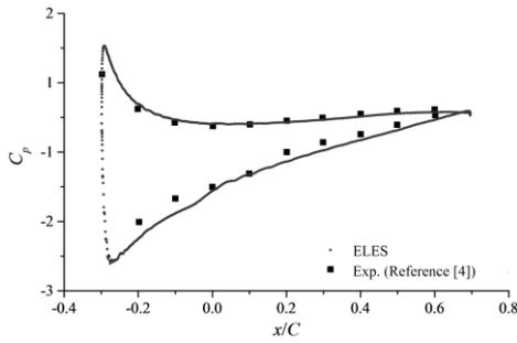
**Fig. 9. Comparison of pressure coefficient between time-averaged ELES and experiments (A0).**
