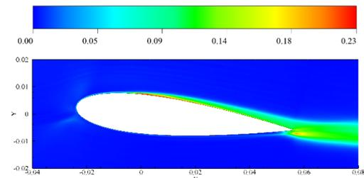
Fig. 8. Streamwise turbulence intensity of case A0 (on  $Z_m$ ).
