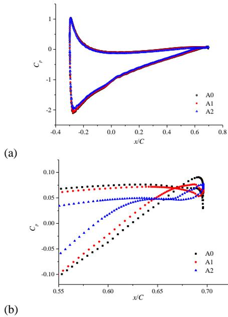
**Fig. 10. Pressure coefficients of airfoils (on Zm).**
