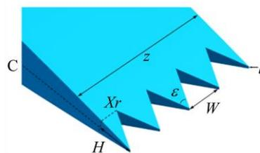
Fig. 1. Geometries of the serrated trailing edge.
