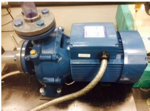
**Fig. 2. Centrifugal pump type F32/200AH.**
