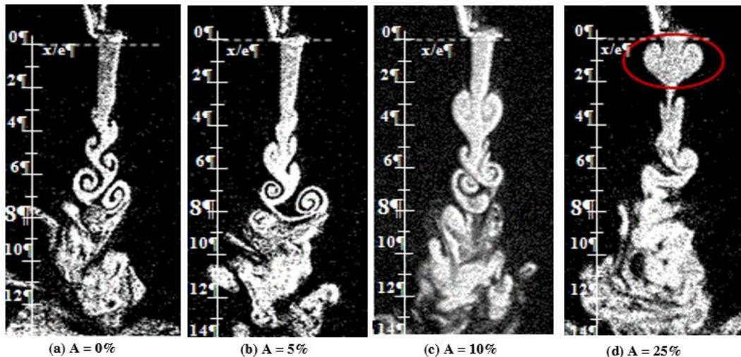
Fig. 6. Pulsation amplitude effect on the jet evolution for  $Re = 500$ , and  $St = 0.1$ .
