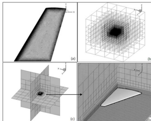
**Fig. 8.** (a) Magnified outlook of the surface grid of the ONERA M6 wing on XY plane, (b) isometric view of the Cartesian grid solution domain around the wing, (c) sliced expression of the whole domain wing-centred, (d) close-up view on the grid.
