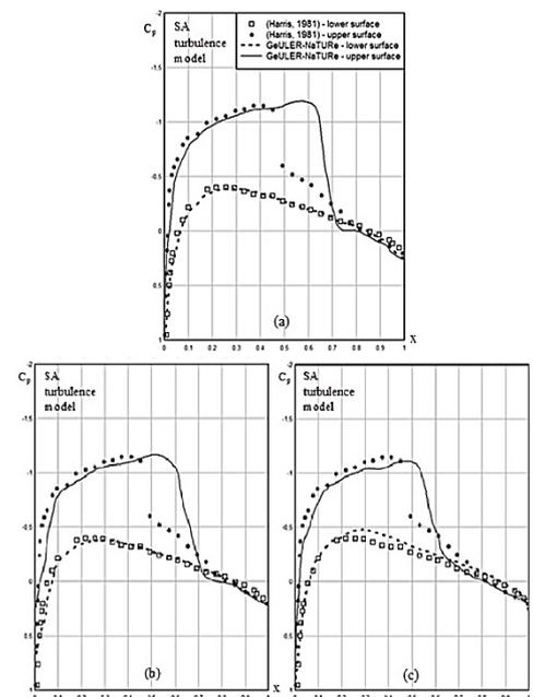
**Fig. 4. Pressure coefficient ( $c_p$ ) distribution results of [Harris \(1981\)](#) compared with GeULER-NaTure around NACA0012 with SA turbulence model having (a) 0.05 units, (b) 0.02 units and (c) 0.01 units;  $M_\infty = 0.799$ ,  $\theta = 2.26^\circ$ ;  $Re = 9 \times 10^6$ .**
