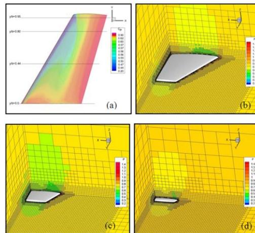
**Fig. 12. Spanwise slices on transonic ONERA M6 wing, (a)  $y/b=0.44$ , (b)  $y/b=0.65$ , (c)  $y/b=0.80$ , (d)  $y/b=0.95$ ;  $M_\infty=0.8395$ ,  $\theta = 3.06^\circ$ , (inviscid, laminar), (Kara *et al.*, 2016).**
