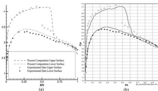
**Fig. 6. Pressure coefficient ( $c_p$ ) distribution of (a) Aybay (2004) compared with (b) GeULER-NaTURE around NACA0012 airfoil with two solution refinements and SA turbulence model with 0.01 units;  $M_\infty = 0.799$ ,  $\theta = 2.26^\circ$ ;  $Re = 9 \times 10^6$ .**
