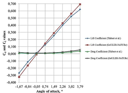
**Fig. 7.**  $C_d$  and  $C_l$  values of Thibert *et al.* (1979) in comparison with GeULER-NaTure turbulent flow solver results around NACA0012 airfoil at eight different angle of attacks having  $M_\infty = 0.75$ ,  $Re = 4 \times 10^6$ .
