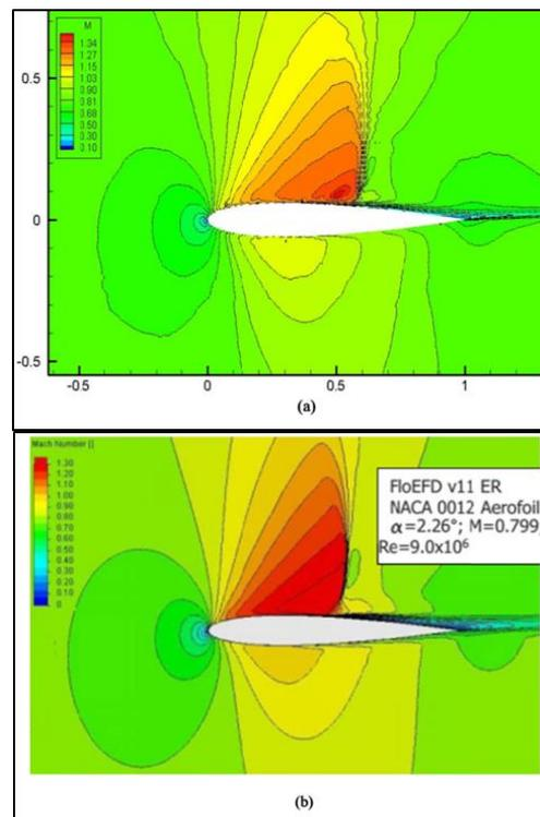
**Fig. 5. Mach number contours of (a) GeULER-NaTURE with SA turbulence model having 0.01 units and (b) FloEFD (Mentor Graphics, 2010) around NACA 0012;  $M_\infty = 0.799$ ,  $\theta = 2.26^\circ$ ;  $Re = 9 \times 10^6$ .**
