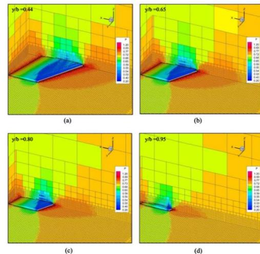
**Fig. 9.** Spanwise slices on transonic ONERA M6 wing, (a)  $y/b=0.44$ , (b)  $y/b=0.65$ , (c)  $y/b=0.80$ , (d)  $y/b=0.95$ ;  $M_\infty=0.8395$ ,  $\theta = 3.06^\circ$ ,  $Re = 11.7 \times 10^6$ , (viscous turbulent).
