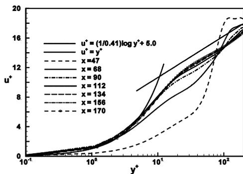
Fig. 17. Streamwise velocity profiles of relaxing boundary-layer for the dynamic model.
