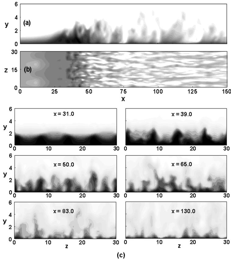
Fig. 11. Contours of instantaneous streamwise velocity: (a) x-y plane at  $z = 30.0$ ; (b) x-z plane at  $y = 0.05$ ; (c) y-z planes at indicated x-locations. Maximum level is 0.98 and minimum level is -0.13.
