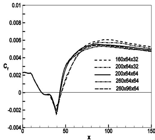
Fig. 3. Evolution of  $C_f$  for different grid levels.
