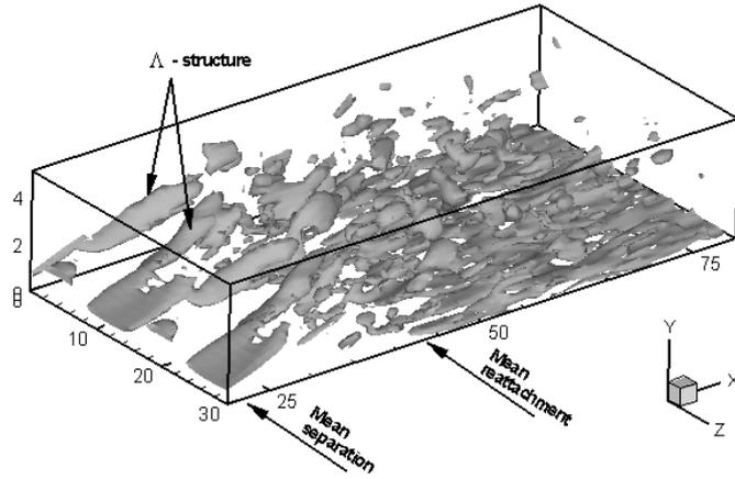
Fig. 13. Iso-surfaces of the spanwise component of instantaneous vorticity. Contour level is -0.55.
