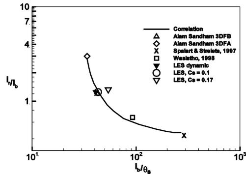
Fig. 19. Bubble length versus the recovery length.
