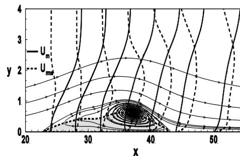
**Fig. 9. LES of a laminar separation bubble showing streamlines,  $u_m$  and  $u_{rms}$ .**
