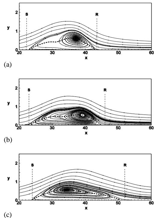
**Fig. 7.** LES of a laminar separation bubble showing streamlines and  $u_m = 0$  line (dashed line) for (a) dynamic model; (b) Smagorinsky model,  $C_s = 0.1$  and (c) Smagorinsky model,  $C_s = 0.17$ .
