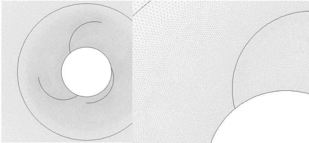
Fig. 7. Computational grid near the turbine blades.
