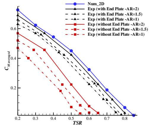
**Fig. 13.** Variations of the experimental averaged torque coefficients, for the 3-bladed rotor at various aspect ratios.
