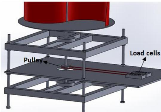
Fig. 3. Schematic of the torque measuring device.
