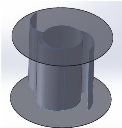
**Fig. 5. A schematic of the rotor with endplates.**
