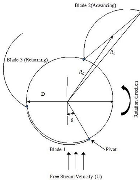
**Fig. 1. Geometrical parameters of a 3-bladed rotor.**
