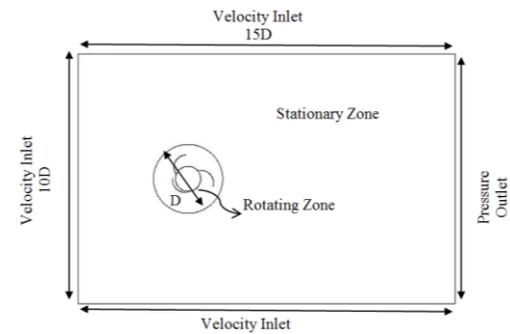
**Fig. 6. Computational domain and the boundary conditions.**
