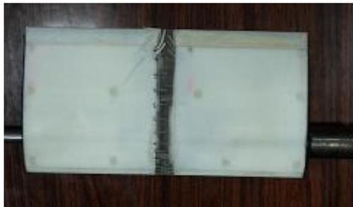
Fig. 2. Fabricated model of the airfoil.
