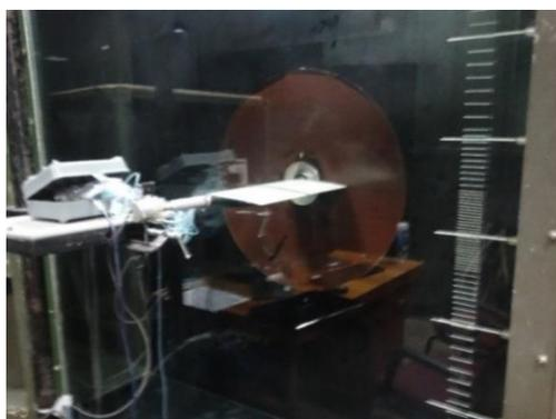
Fig. 3. NACA 0012 airfoil model mounted in the wind tunnel with instrumentation for pressure acquisition.
