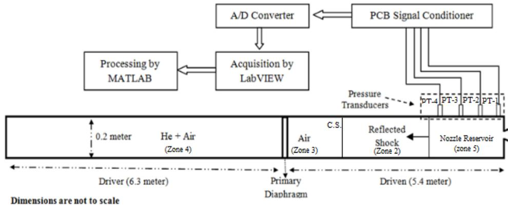
**Fig. 1. Schematic illustration of the shock tube facility.**
