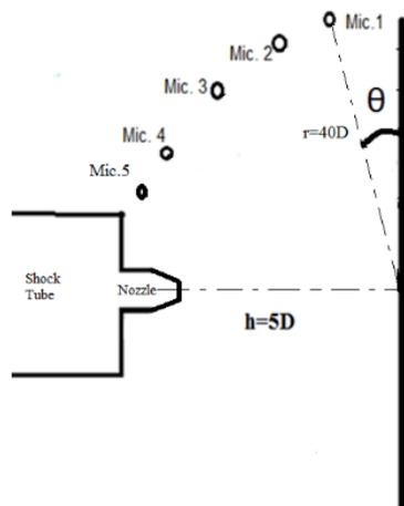
**Fig. 9. Position of the microphones for normal jet impingement.**
