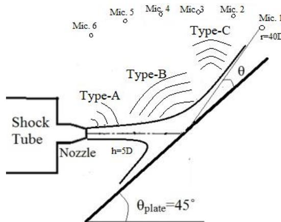
**Fig. 5.** Position of the microphones at the oblique jet impingement to a  $45^\circ$  inclined plate.
