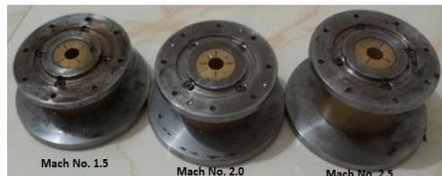
**Fig. 6. Fabricated nozzles for Mach numbers 1.5, 2.0 and 2.5.**
