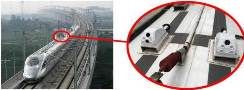
**Fig. 1. Train pantograph network monitoring device.**
