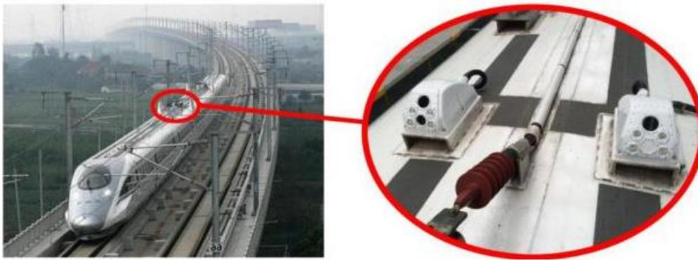
**Fig. 1. Train pantograph network monitoring device.**
