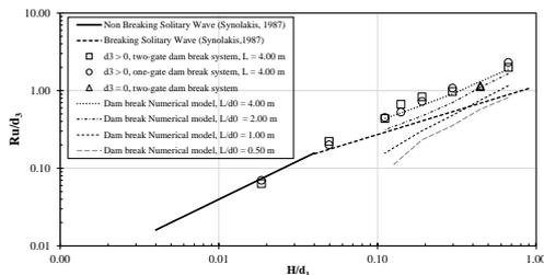
**Fig. 11. Surge run-ups of the numerical model as compared with those from the present physical model and [Synolakis \(1987\)](#).**
