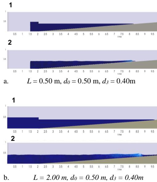
**Fig. 12. Numerical dam break waves propagation using DualSPHysics. (1) Initial condition, (2) After 8.50 s.**
