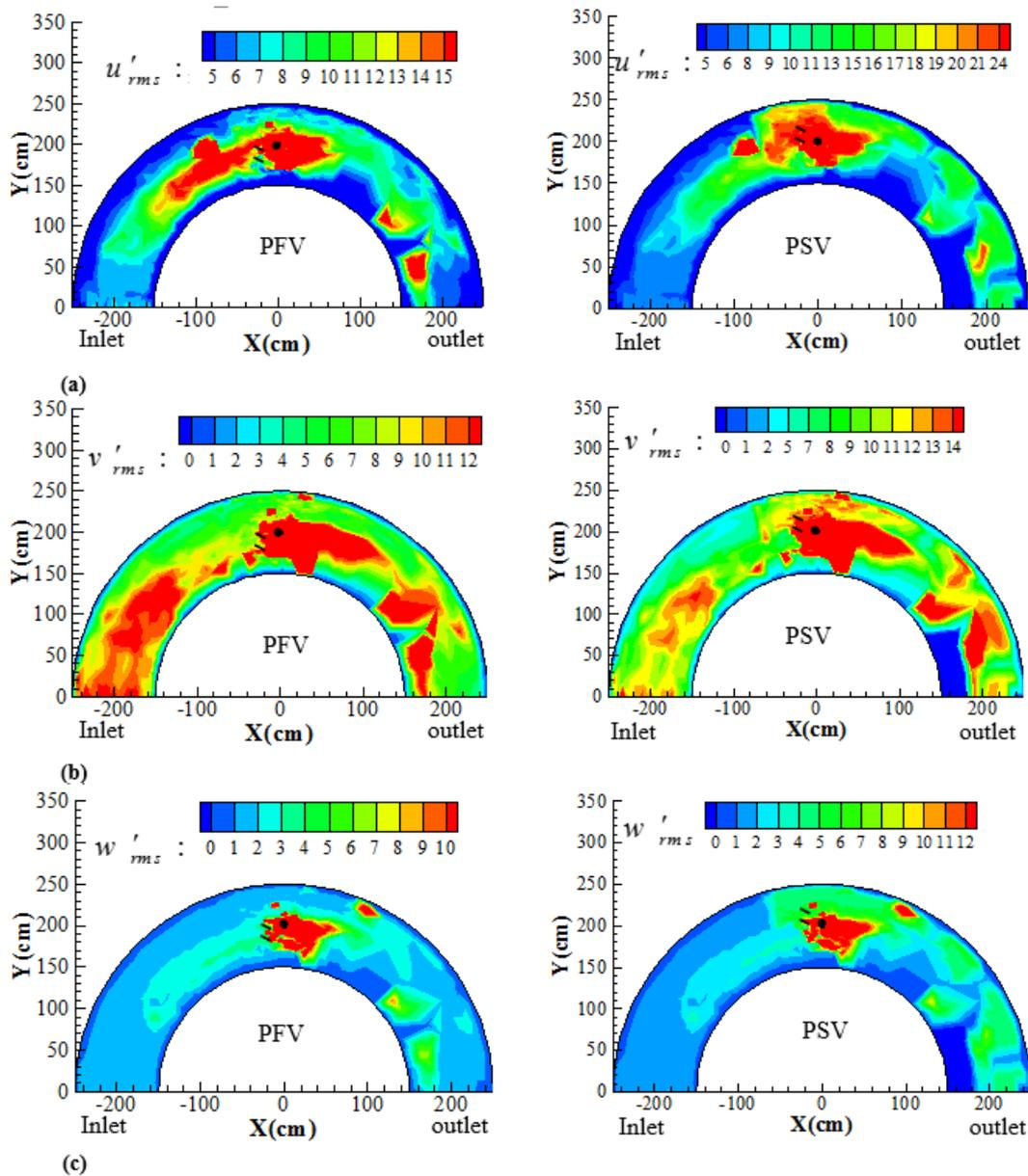
**Fig. 5. Distribution of flow turbulence intensities ( $cm/s$ ) in the 180 degree sharp bend at a level equal to 5% of the flow depth from the bed in (a) longitudinal  $u'_{rms}$ , (b) transverse  $v'_{rms}$ , and (c) vertical  $w'_{rms}$  directions.**
