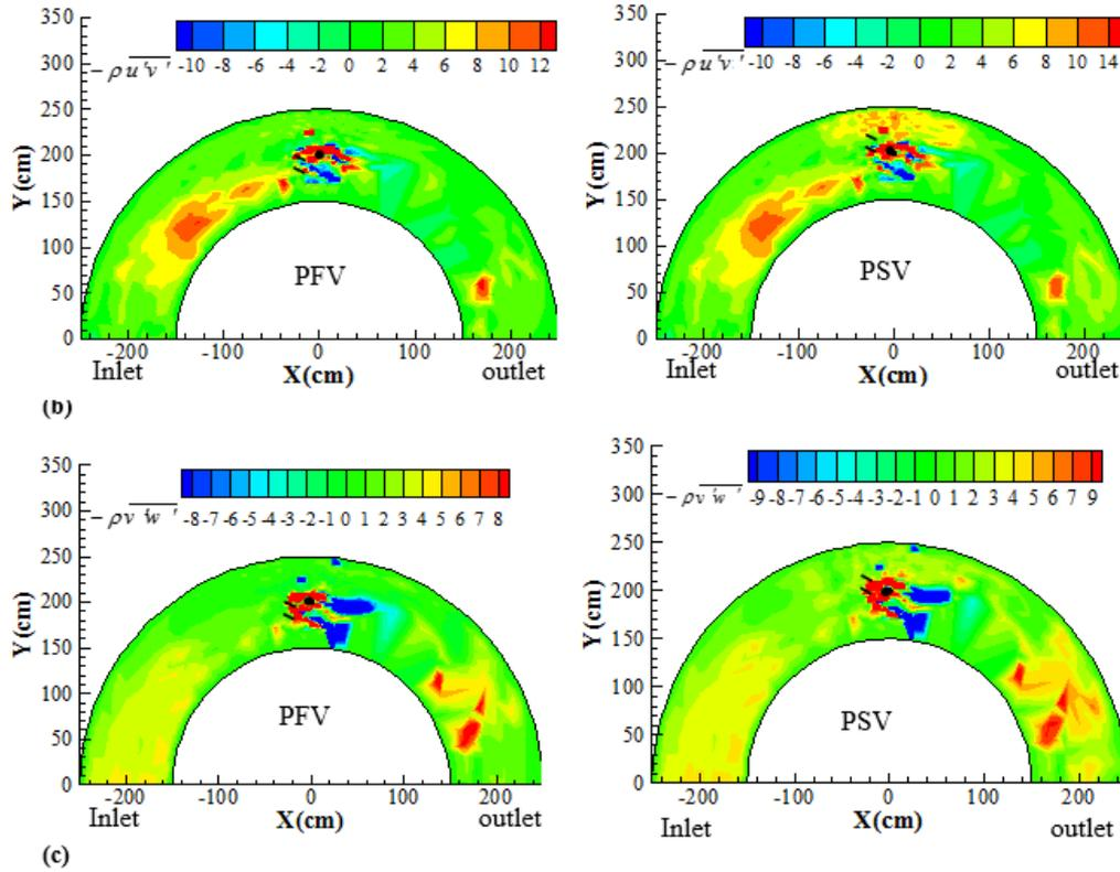
**Fig. 8. Bed shear stress distribution ( $gr / cm \times s^2$ ) in the 180 degree sharp bend at a level equal to 5% of the depth from the bed in (a) longitudinal, (b) transverse, and (c) vertical directions.**
