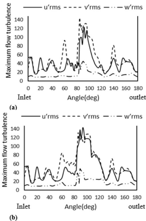
**Fig. (6).** Distribution of the maximum flow turbulence intensities (*cm / s*) in longitudinal, transverse, and vertical directions in (a) PFV, and (b) PSV experiments.
