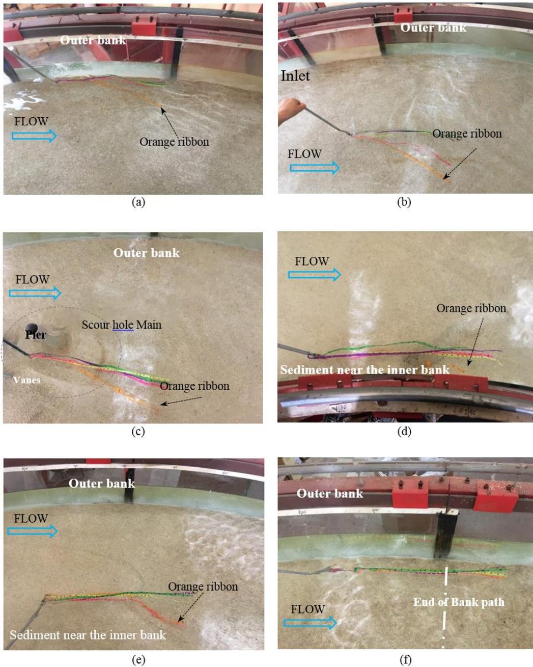
**Fig. 10.** A view of the qualitative flow pattern using orange ribbons at different cross sections in the 180 degree sharp bend at (a) 25, (b) 55, (c) 90, (d) 135, (e) 155 degrees, and (f) the end of the bend.
