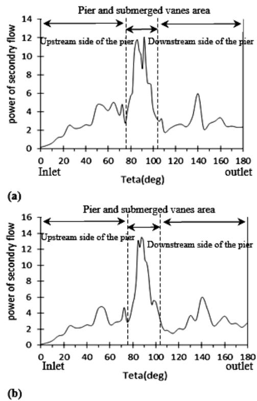
**Fig. 7.** Diagrams on the secondary flow strength throughout the bend in (a) PFV and (b) PSV experiments.
