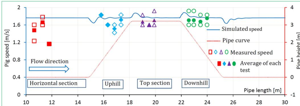
Fig. 6. Pig speed of the measurement vs. the speed of the simulation.
