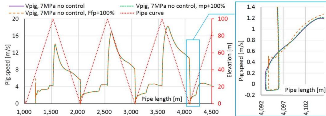
Fig. 13. Pig speeds vs. Pipe length (the mass or the contact force of the pig is doubled).
