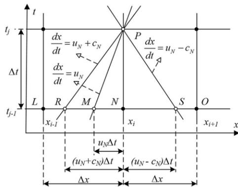
Fig. 3. Characteristics used in MOC.
