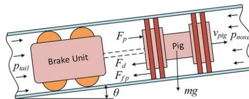
Fig. 1. Pig carries a brake unit in pipeline.
