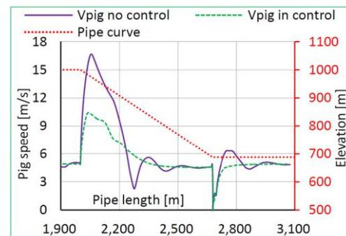
Fig. 15. Pig speed in control vs. no control.
