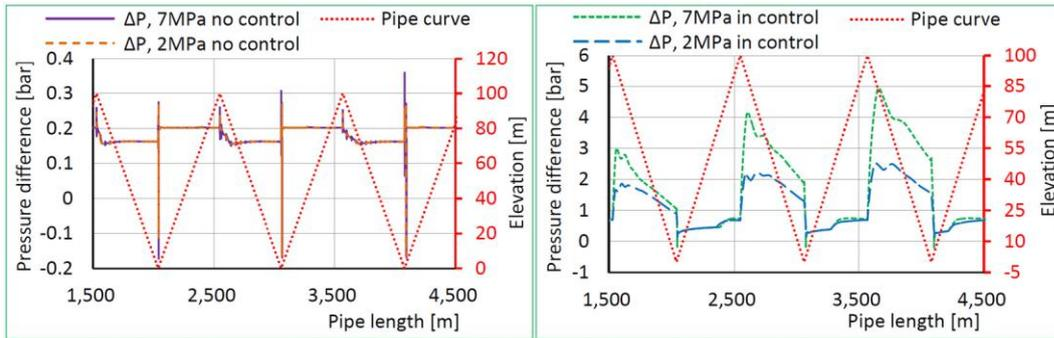
Fig. 9. Pressure difference between pig tail and nose.
