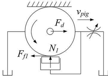
**Fig. 2. Schematic principle of the brake unit.**
