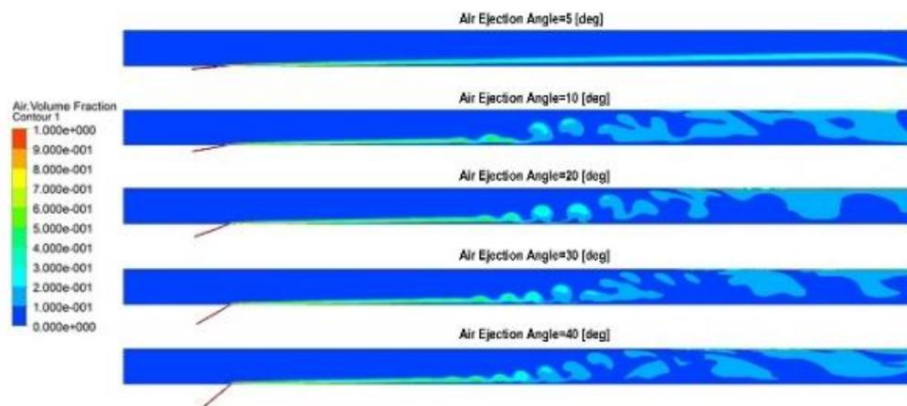
Fig. 8. Flow regime under different air ejection angles ( $V_a=2 \text{ m}\cdot\text{s}^{-1}$ ,  $\text{time}=30 \text{ s}$ ).
