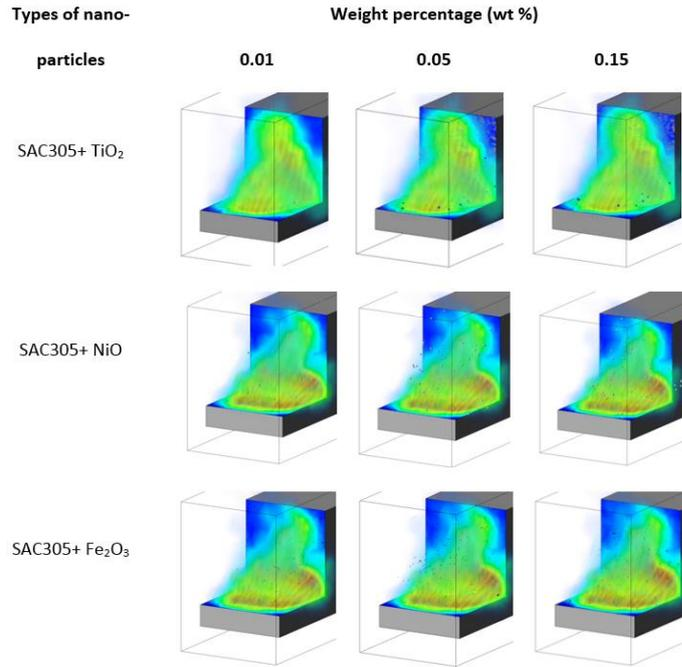
Fig. 7. 3D model-view of wetted SAC305 with nanoparticles.
