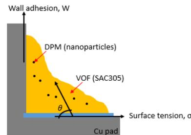
**Fig. 5. Schematic diagram of boundary condition.**
