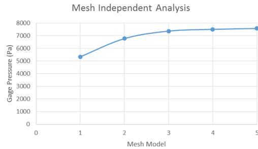
Fig. 2. Mesh independent analysis graph.
