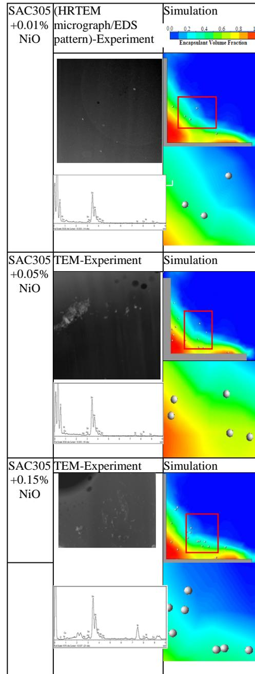
**Fig. 10. Comparison of the NiO nanoparticle distribution between simulation and experimental results.**
