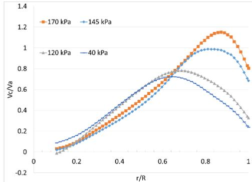
**Fig. 8. Effect of injection pressure on induced vortex.**
