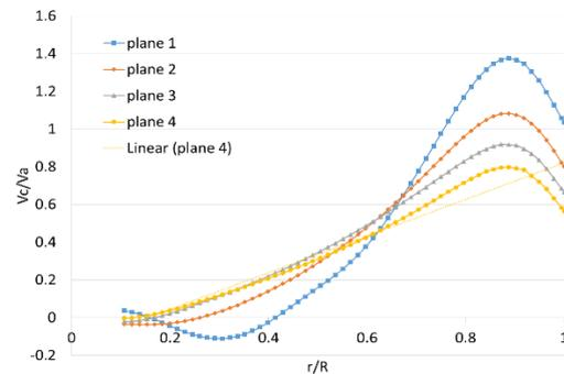
**Fig. 7. Normalized circumferential velocity distribution along the tube.**
