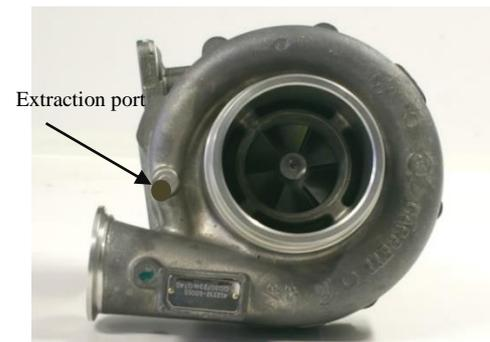
**Fig. 12. Extraction point for supply of high pressure injection air.**
