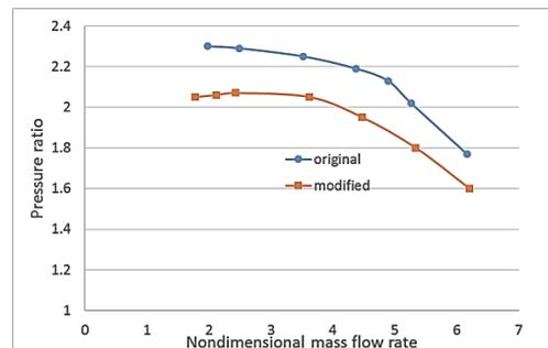
**Fig. 16. Pressure ratio comparison of the original and modified compressor.**
