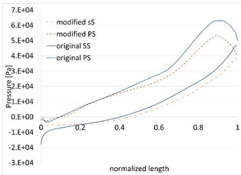
**Fig. 19. Pressure loading on main blades near surge.**
