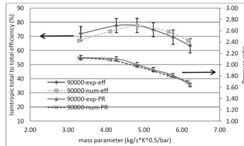
**Fig. 11. Numerical and experimental performance of the compressor at 92krpm.**
