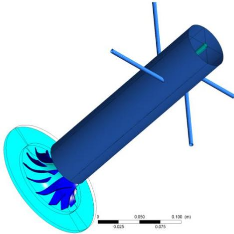
**Fig. 13. Model of the compressor and the inlet assembly.**
