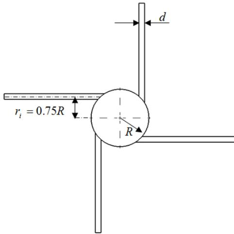
**Fig. 5. Adjusted positions of the injectors.**
