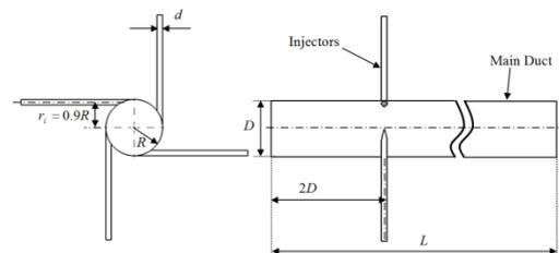
Fig. 2. Injectors and the main duct locations.
