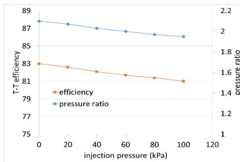
**Fig. 14. Injection pressure effect on compressor performance at nominal point.**
