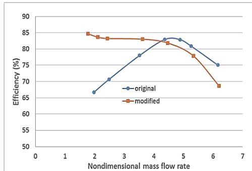
**Fig. 17. Efficiency comparison of the original and modified compressor.**
