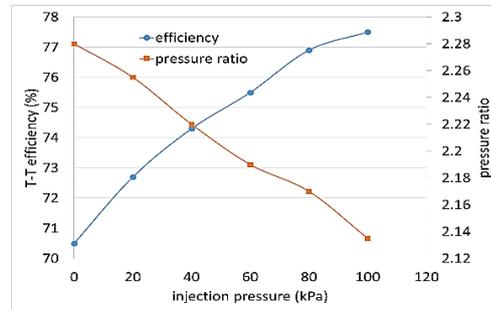
**Fig. 15. Injection pressure effect on compressor performance at low mass flow rates.**
