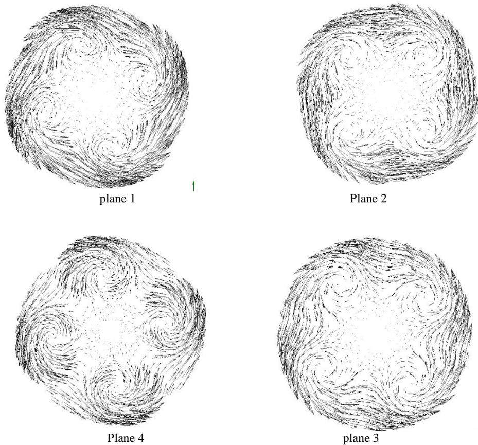
**Fig. 4. Vectors of circumferential velocity along the tube for the tangential case ( $r_i=0.9R$ ).**
