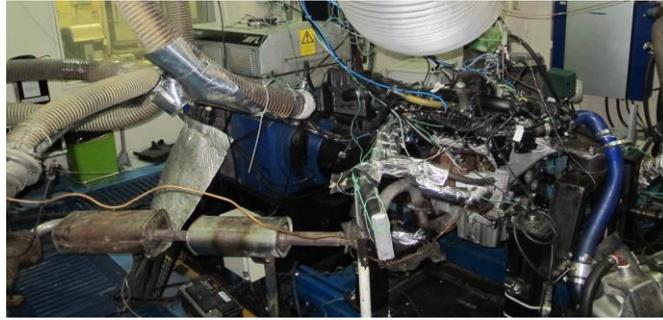
Fig. 3. AVL APA 1F4-E-0509 dynamometer and other accessories.
