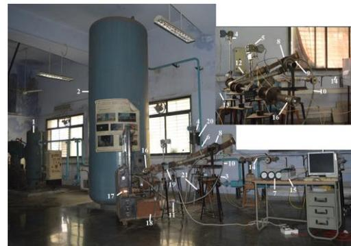
(1- compressor, 2- air receiving tank, 3- PRV, 4, 5- flow meters, 6- pressure tapping, 7- pressure gauge, 8- test turbine, 9- load compressor, 10- cooling oil in, 11- cooling oil out, 12- spark electrode, 13- fuel supply, 14- thermocouples, 15- data logger, 16- load valve, 17- cooling oil pump, 18- cooling oil tank, 19- flow totalizer, fuel supply tank, 21- fuel pump assembly)
