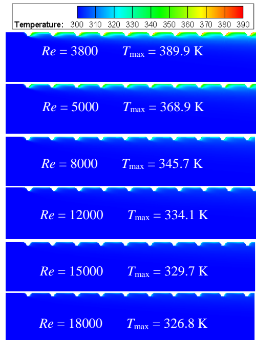
Fig. 12. Static temperature contours for e/D=.042 and p/e=7.14 for different Re number.
