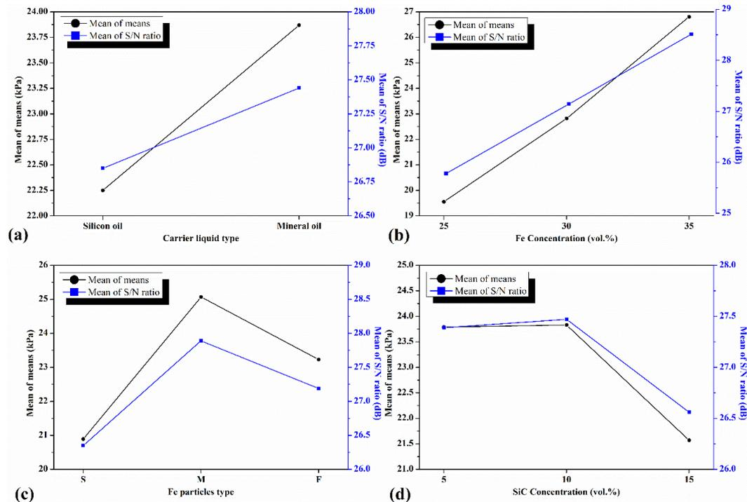
**Fig. 8. Main effects plot for Mean of means and Mean of S/N ratio.**
