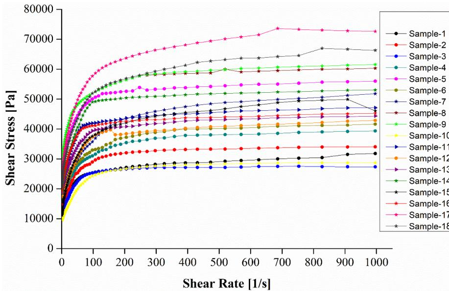
Fig. 4. Flow curves of all the 18 samples at a magnetic field strength of 0.6 T.
