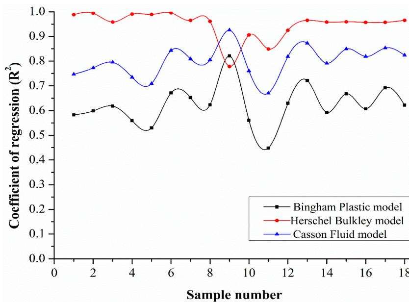
Fig. 5. Coefficient of regression of all the samples as per BP, HB and Casson fluid models.
