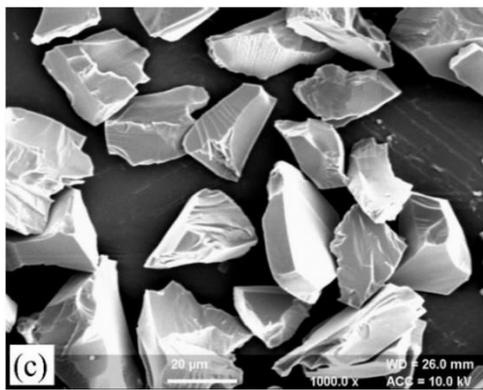
**Fig. 1.** SEM micrograph of (a) spherical iron particles (b) flake type iron particles and (c) abrasive (SiC) particles.
