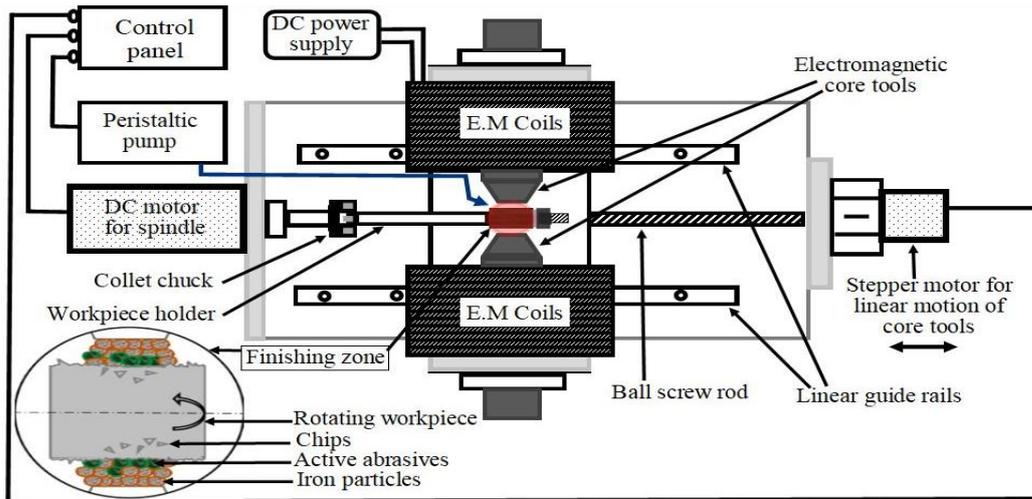
**Fig. 10.** Schematic of the used MR fluid finishing process.
