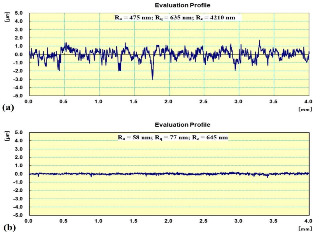
**Fig. 11. Surface roughness profile of SS316L workpiece (a) before finishing and (b) after finishing with optimized fluid sample.**
