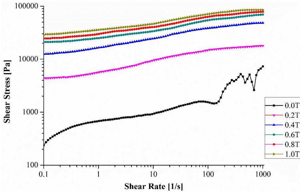
**Fig. 9.** Yield stress of optimized fluid sample at different magnetic field strengths.
