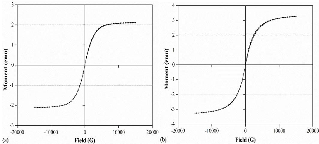
**Fig. 2. VSM spectra of (a) spherical type iron particles and (b) flakes type iron particles.**
