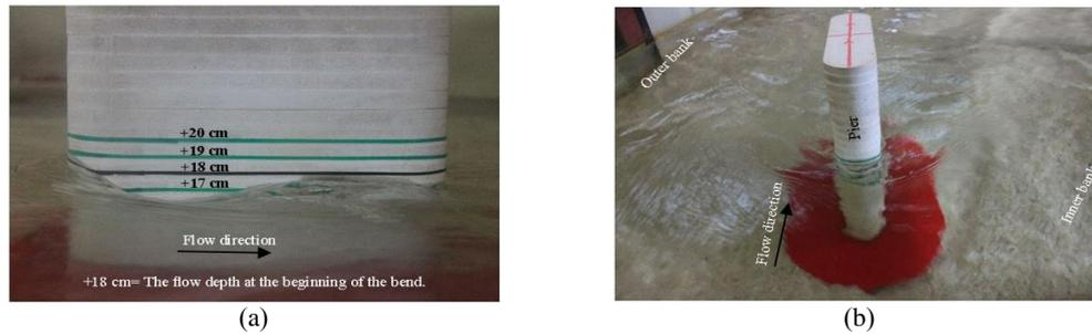
**Fig. 10. Flow pattern around the pier a) View of the inner bank and b) Pier nose.**
