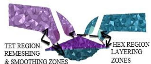
**Fig. 7. Volume Discretization of different parts.**
