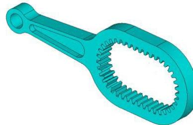
**Fig. 2. Proposed connecting rod.**
