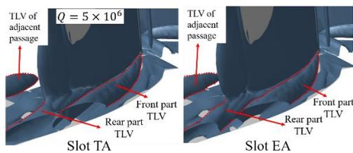
Fig. 21. Q-Isosurface of BTS.
