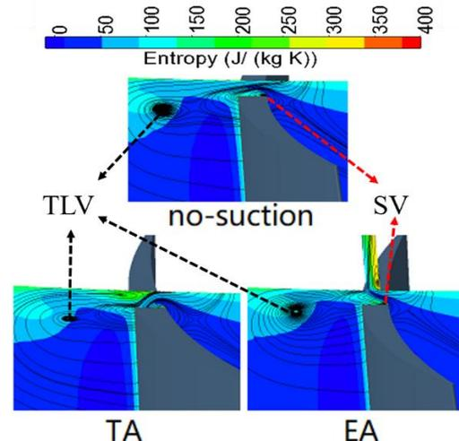
Fig. 19. Streamlines/entropy contour on 40% chord slices with SFR of 0.5%.
