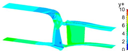
**Fig. 2. Distribution of dimensionless wall distance.**
