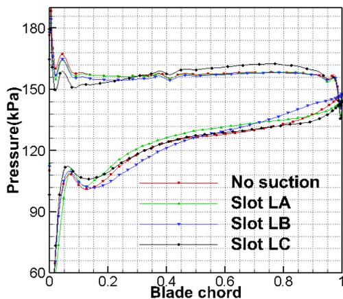
Fig. 15. Static pressure distribution of 5% span in the stator blade.
