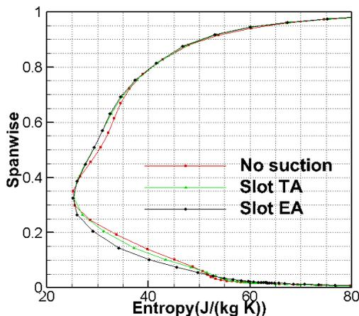
Fig. 23. The entropy distribution at stator outlet.
