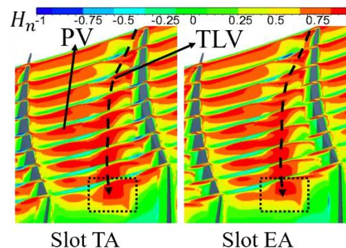
Fig. 20. The normalized helicity on different axial slices of TS with SFR of 0.5%.
