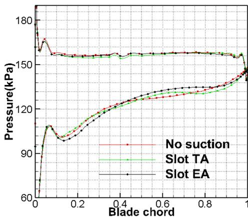
Fig. 22. Static pressure distribution of 5% span.
