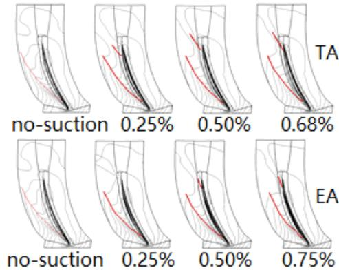
Fig. 17. Static pressure contour distribution on the end wall of the stator hub.
