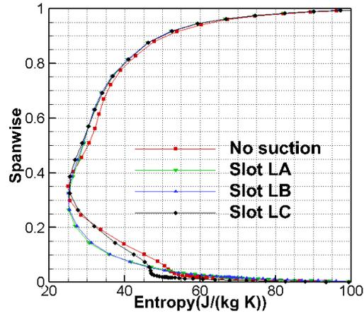
Fig. 16. Circumferential average entropy distribution of the stator exit.
