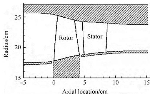
Fig. 1. Structure of the axial single-stage transonic compressor.
