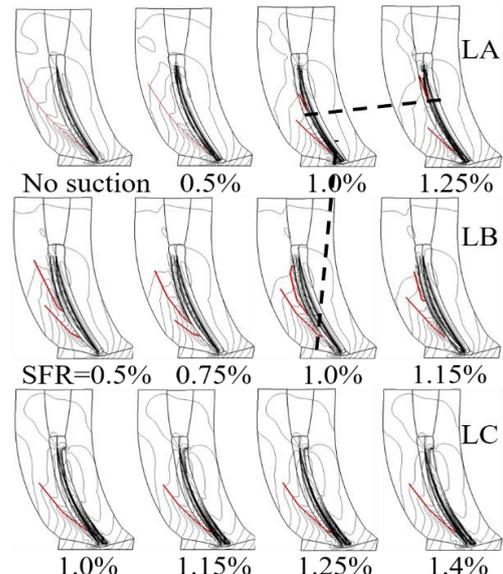
**Fig. 10. Static pressure isolines of the endwall.**
