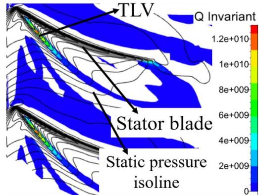
**Fig. 9. Q Invariant and static pressure isolines of original stator passage.**
