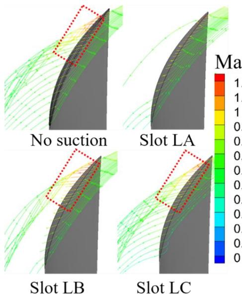
Fig. 11. Three-dimensional streamlines of TLV with SFR of 1.0%.
