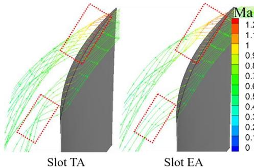
Fig. 18. 3D streamlines of the TLF with an SFR of 0.5%.
