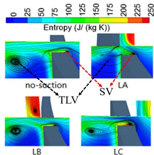
Fig. 12. Streamlines/entropy contour on 35% axial chord slices with SFR of 1.0%.
