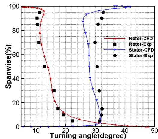
**Fig. 4. Comparison of calculated and experimental flow turning angle at design speed with a mass flow of 20.13kg/s.**
