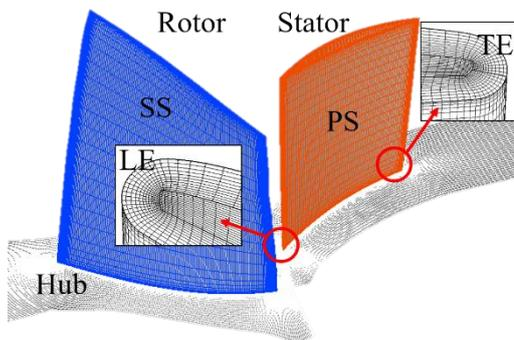
**Fig. 3. Computational mesh of compressor and local enlargement of mesh at the stator blade tip.**
