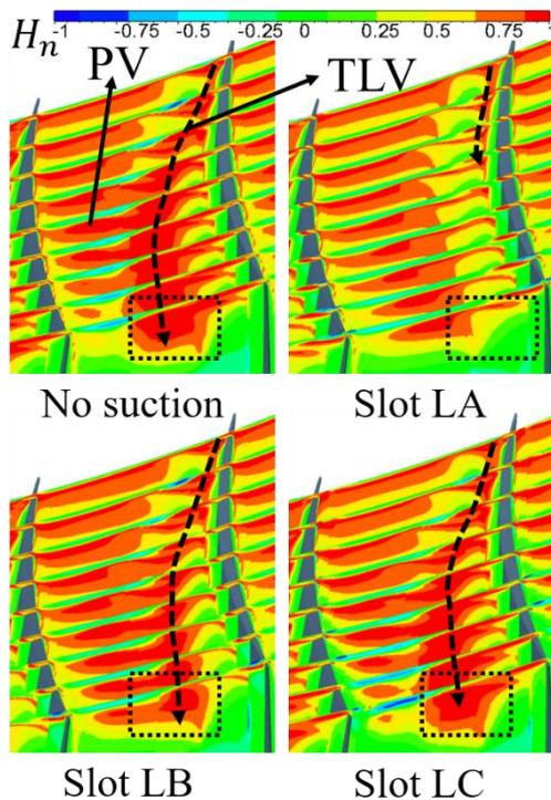
Fig. 13. The normalized helicity on different axial slices of ES with SFR of 1.0%.
