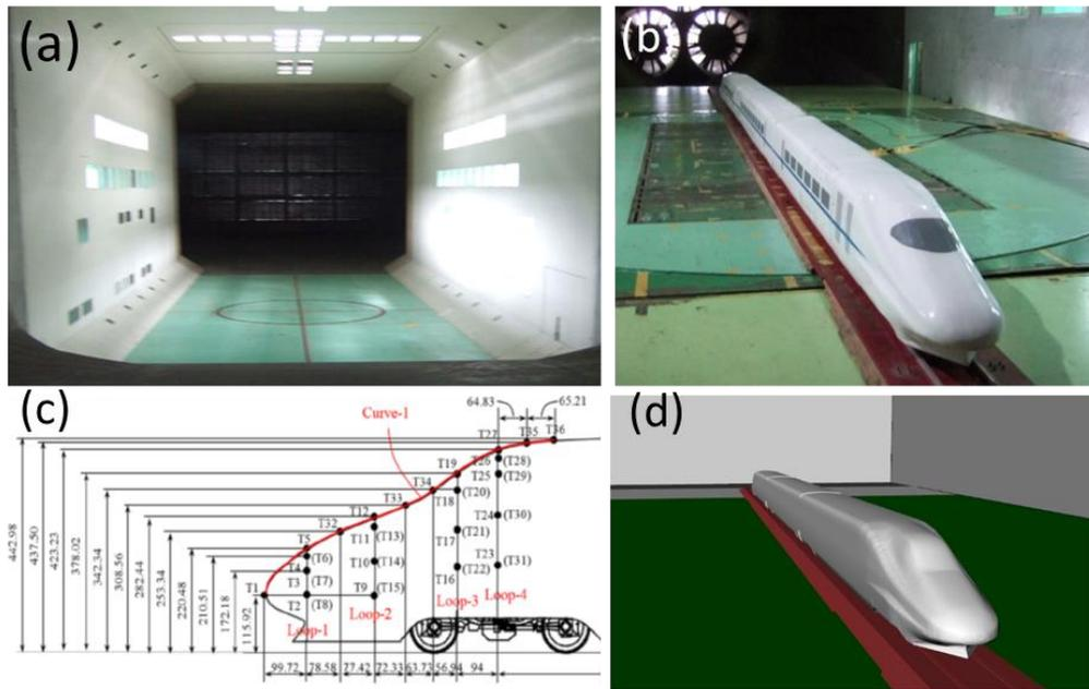
**Fig. 6.** Wind tunnel tests: (a) test section of the wind tunnel; (b) the CRH2 train and rail models; (c) positions of the monitor sensors; (d) simulation under equivalent conditions.
