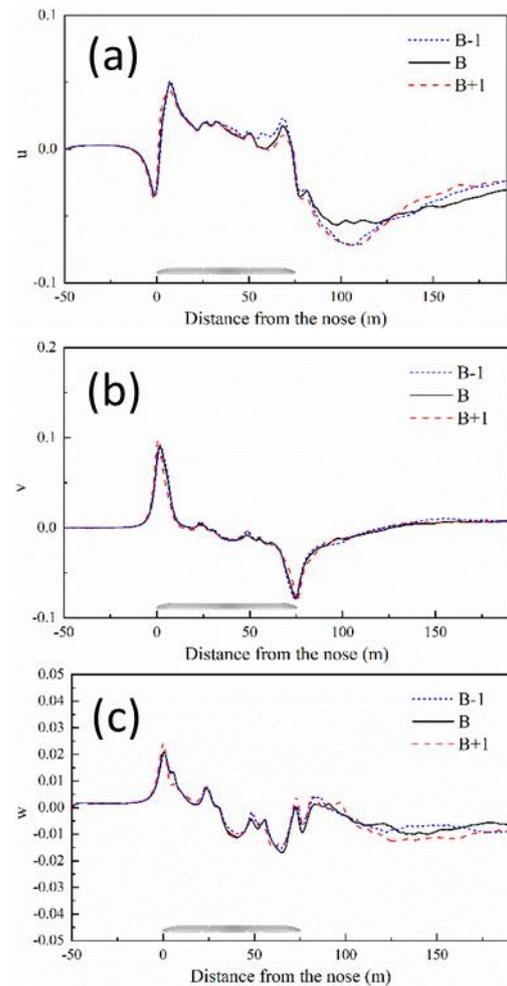
**Fig. 13. Time-averaged magnitudes of the normalized velocity components for the different train models at 3.0 m from the COT and 1.44 m from the TOR: (a) longitudinal velocity,  $u$ ; (b) lateral velocity,  $v$ ; (c) vertical velocity,  $w$ .**
