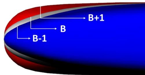
**Fig. 1. Horizontal nose profiles of the high-speed train models employed in the present work.**
