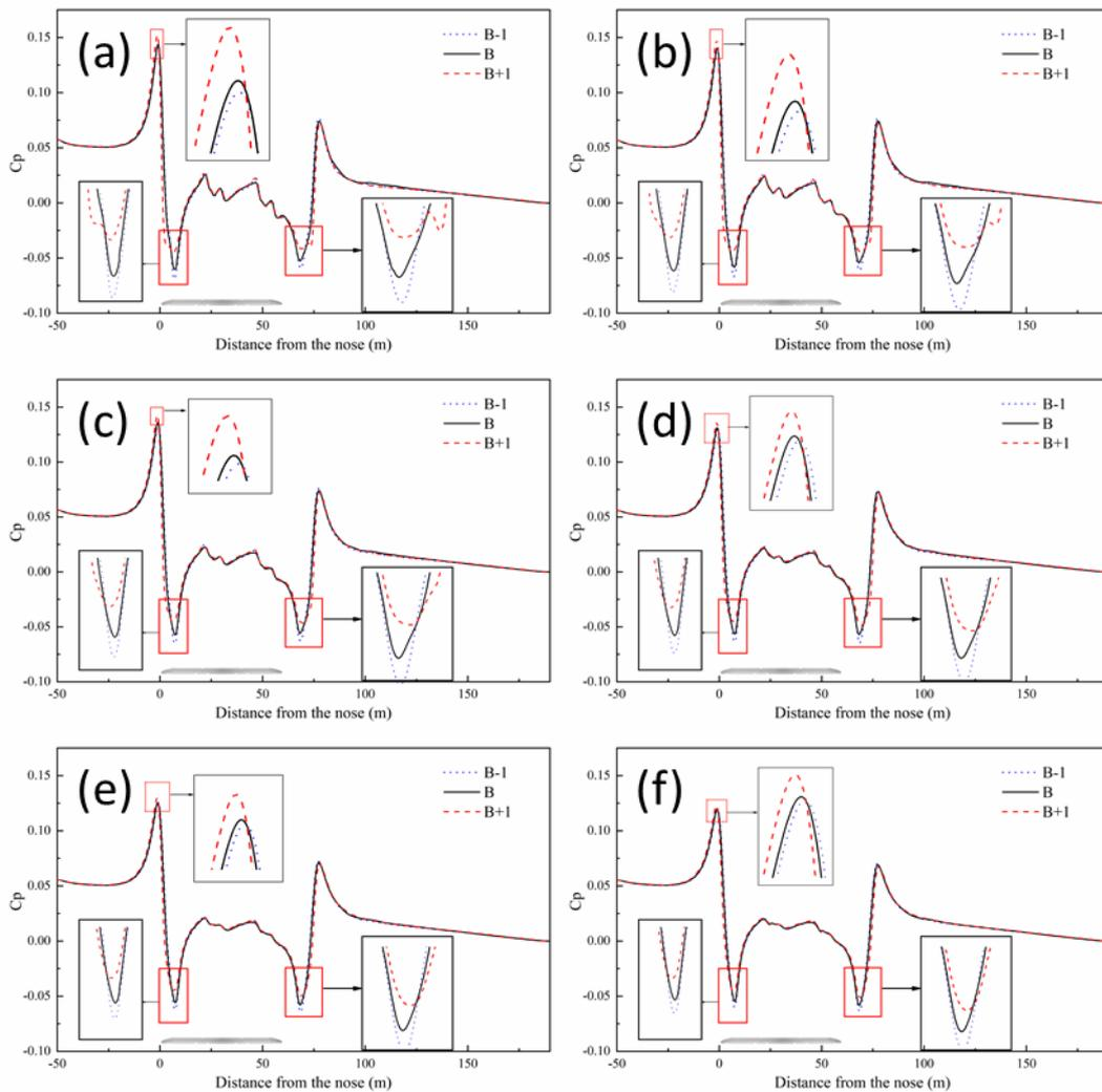
**Fig. 15.** Time-averaged pressure coefficients ( $c_p$ ) of the three train models at  $y = 2.5$  m (i.e., distance from the COT) and at  $z$  values (i.e., distance from the TOR) of (a) 1.5 m, (b) 1.8 m, (c) 2.1 m, (d) 2.4 m, (e) 2.7 m, and (f) 3.0 m.
