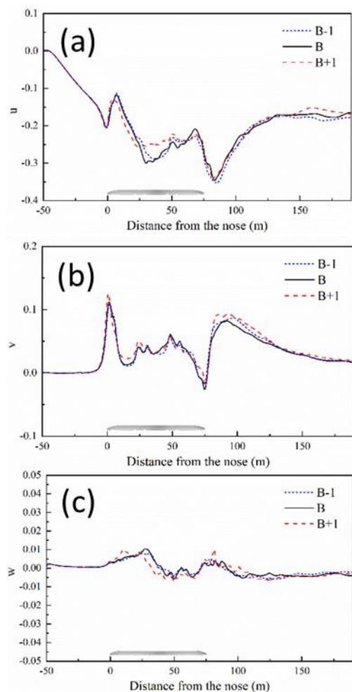
**Fig. 11. Time-averaged magnitudes of the normalized velocity components for the different train models at 3.0 m from the COT and 0.2 m from the TOR: (a) longitudinal velocity,  $u$ ; (b) lateral velocity,  $v$ ; (c) vertical velocity,  $w$ .**
