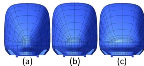
**Fig. 2. Front views of the different high-speed train nose shapes: (a) B-1; (b) B; (c) B+1.**
