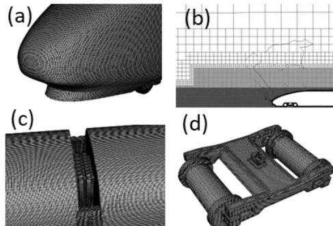
**Fig. 5. Computational mesh employed in the simulations: (a) mesh distribution around the head car; (b) varying mesh density in the computational domain; (c) mesh distribution around the gap; (d) mesh distribution at the bogie.**
