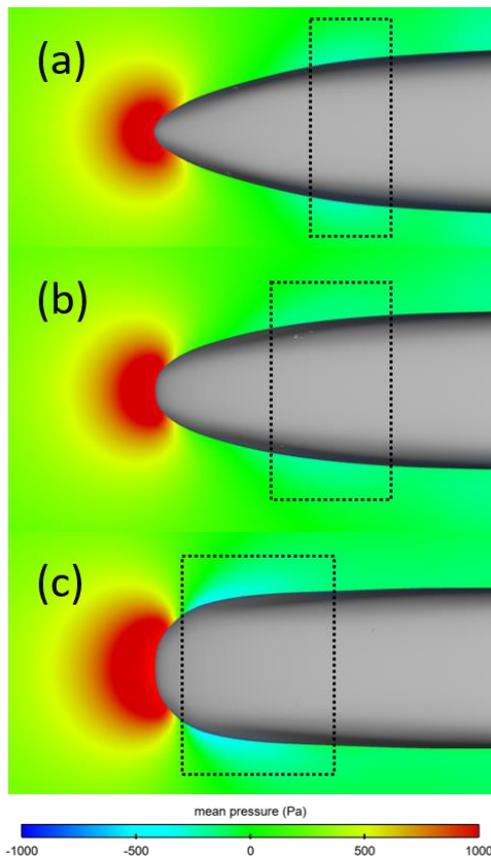
**Fig. 16. Pressure distributions around the three train models within a horizontal plane at 1.5 m from the TOR: (a) B-1; (b) B; (c) B+1.**
