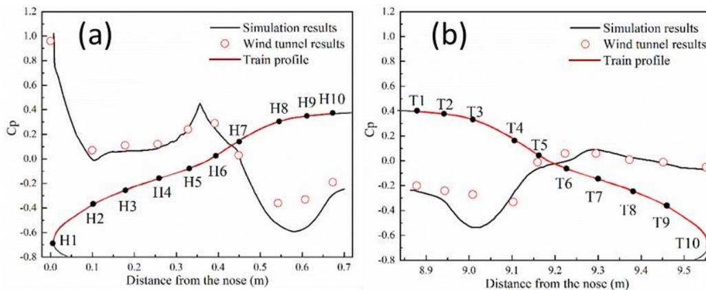
**Fig. 7.** Comparison of calculated and experimental results of the pressure coefficient ( $c_p$ ) on the train surface with respect to the distance from the nose: (a) at curve 1 on the head car; (b) at a symmetrical curve on the tail car.
