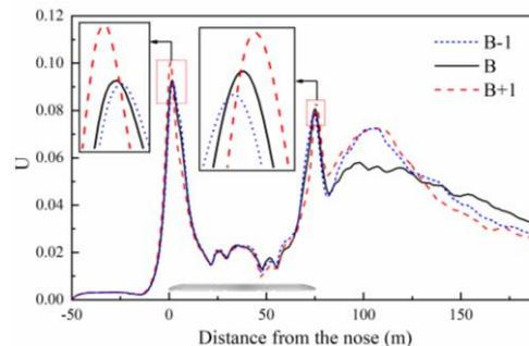
**Fig. 12. Time-averaged values of  $U$  for the different train models at 3.0 m from the COT and 1.44 m from the TOR.**
