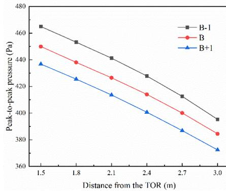
**Fig. 14.** Peak-to-peak pressure values around the nose ( $y = 2.5$  m) of the three train models.
