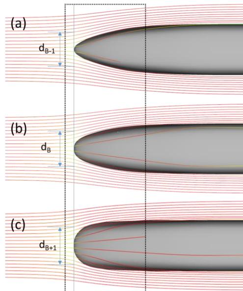
Fig. 10. Streamlines around the three train models within a horizontal plane located at 1.44 m from the TOR: (a) B-1; (b) B; (c) B+1.
