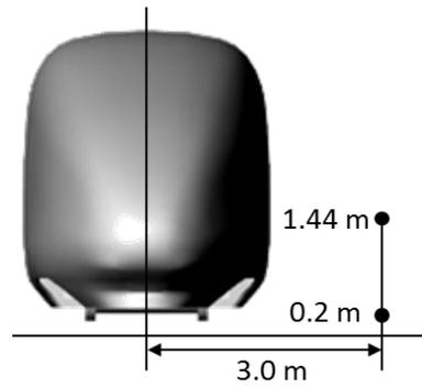
Fig. 8. Positions of points required by the EN standard for measuring  $U$ .
