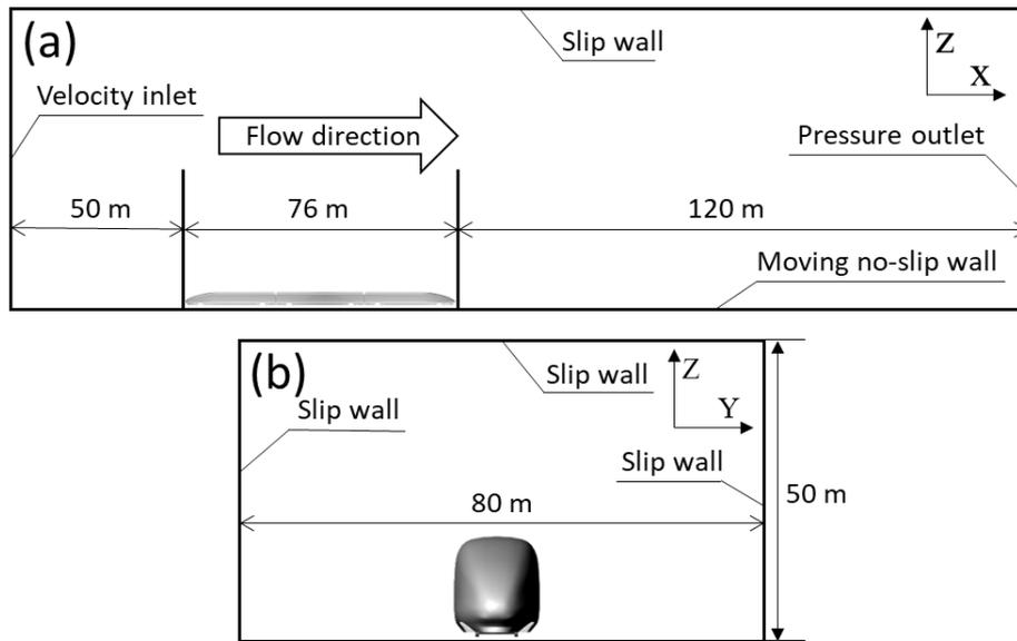
**Fig. 3. Computational domain and boundary conditions: (a) side view; (b) front view.**
