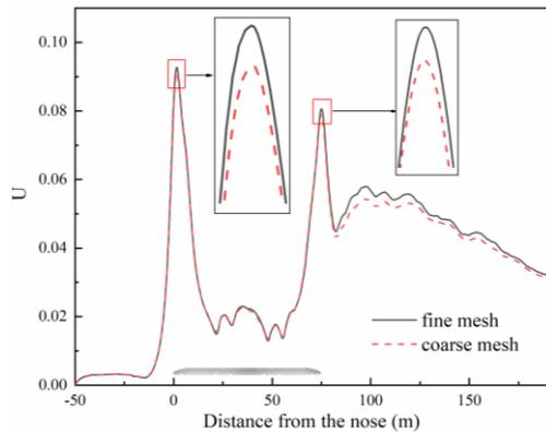
**Fig. 4. Mesh sensitivity of the time-averaged magnitude of the normalized velocity of the slipstream ( $U$ ) for coarse and fine meshing with respect to the distance from the nose of the head car.**
