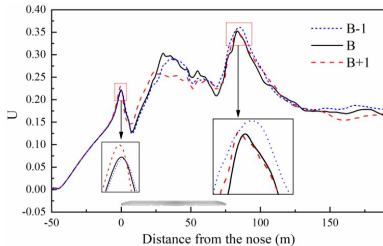
Fig. 9. Values of  $U$  for the different train models at 3.0 m from the COT and 0.2 m from the TOR with respect to the distance from the nose.
