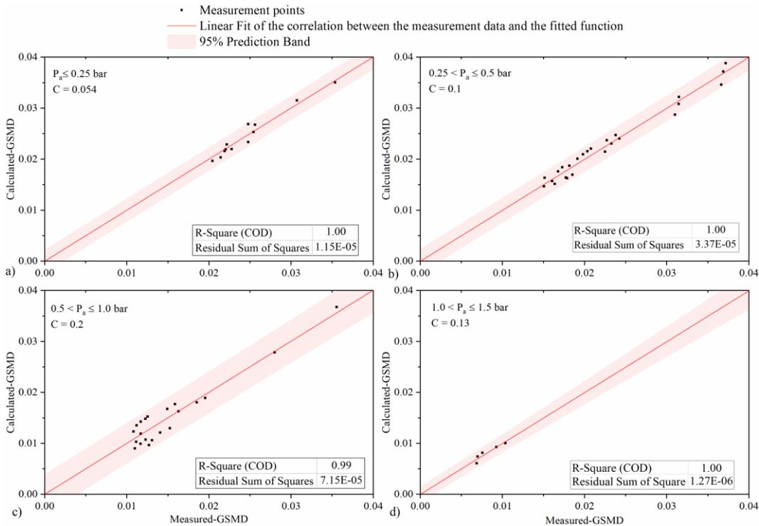
**Fig. 14. Predicted versus experimental dimensional droplet diameters for the prefiling airblast atomizers at different air pressure ranges. a) P<sub>a</sub> ≤ 0.25 bar, b) 0.25 < P<sub>a</sub> ≤ 0.5 bar, c) 0.5 < P<sub>a</sub> ≤ 1.0 bar and d) 1.0 < P<sub>a</sub> ≤ 1.5 bar.**
