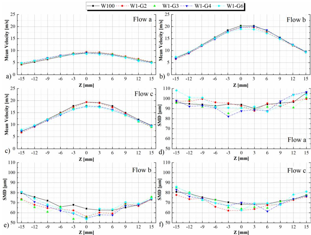
**Fig. 7. Influence of the liquid viscosity on the mean velocity (a, b and c) and SMD (d, e, and f) along the radial direction.**
