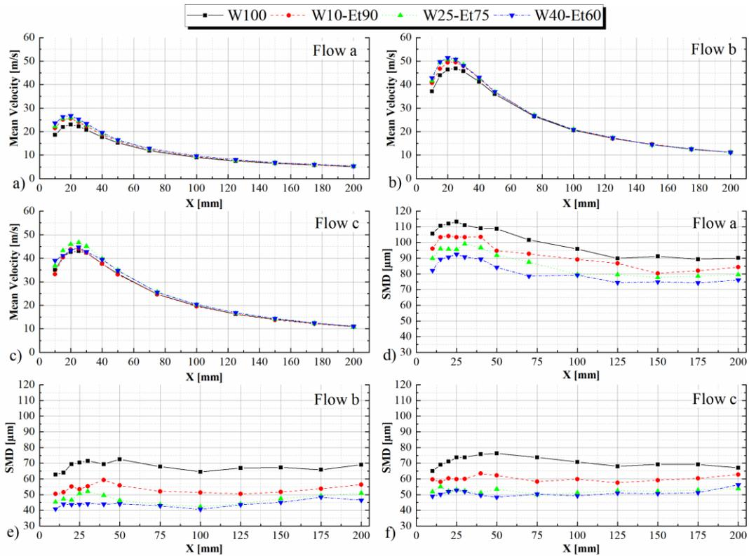
**Fig. 11.** Influence of the liquid surface tension on mean velocity (a, b and c) and SMD (d, e, and f) along axial direction.
