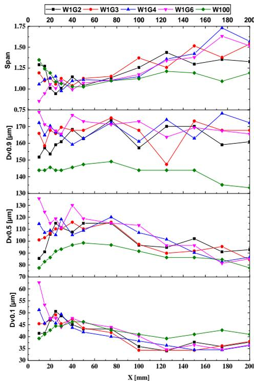
**Fig. 9. Influence of the viscosity on  $D_{0.1}$ ,  $D_{0.5}$ ,  $D_{0.9}$  and span of the spray ( $P_a = 0.6$  bar and  $Q = 50$  ml/min).**
