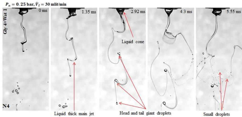
Fig. 4. High viscous liquid breakup in a low-pressure streaming air.
