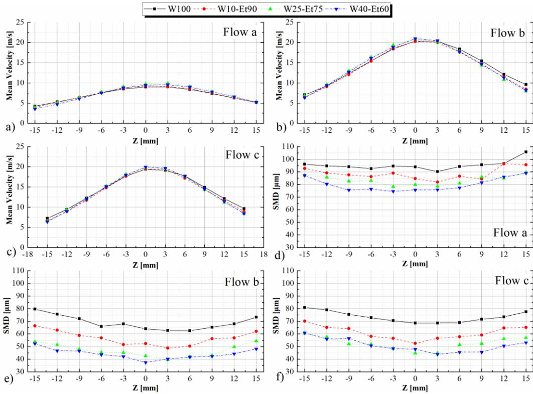
**Fig. 10.** Influence of the liquid surface tension on mean velocity (a, b and c) and SMD (d, e, and f) along radial direction.
