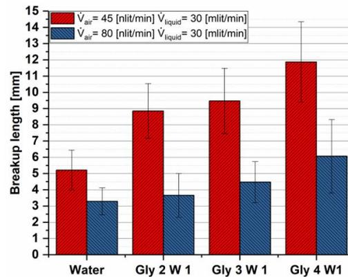
Fig. 6. Influence of the liquid viscosity on the breakup length.
