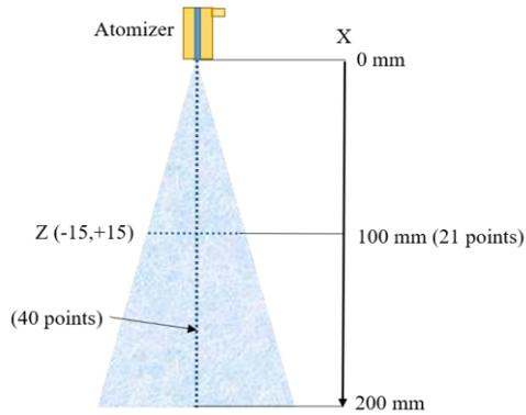
**Fig. 2. PDA measurement locations.**
