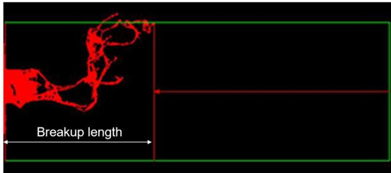
Fig. 5. Breakup length measurement using image processing.
