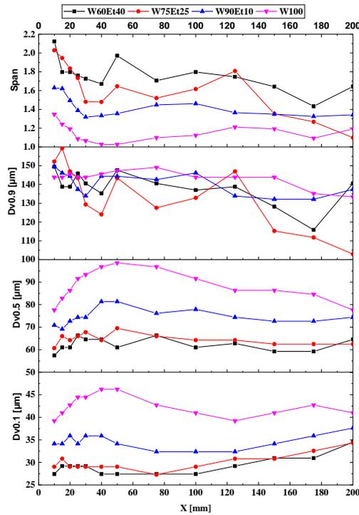
**Fig. 12.** Influence of the surface tension on  $D_{0.1}$ ,  $D_{0.5}$ ,  $D_{0.9}$  and span of the spray ( $P_a = 0.6$  bar and  $Q = 50$  ml/min).
