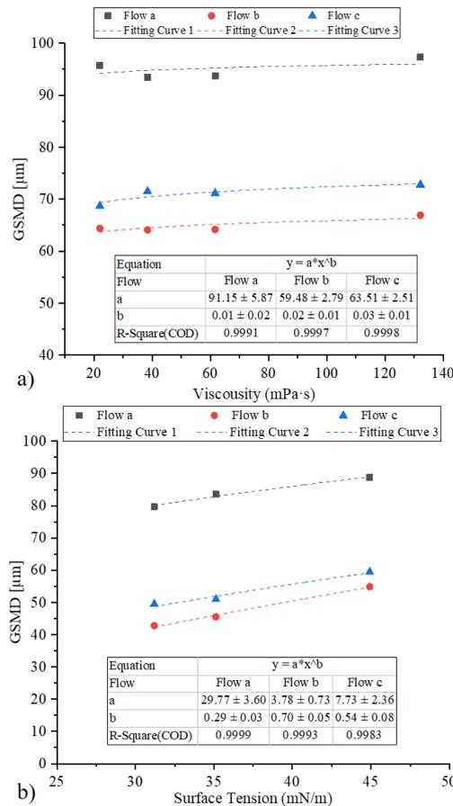
**Fig. 13.** The effect of (a) viscosity and (b) surface tension on GSMD at three different operation conditions (Table 3).
