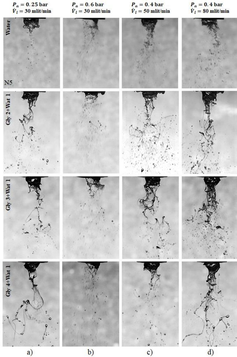
Fig. 3. Effect of the liquid viscosity on the liquid jet breakup mechanism at different operation conditions.
