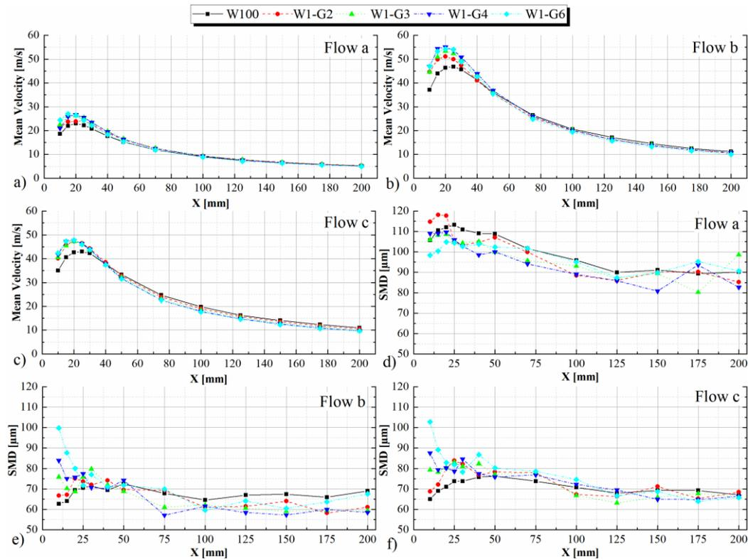
**Fig. 8.** Influence of the liquid viscosity on the mean velocity (a, b and c) and SMD (d, e, and f) along the axial direction.
