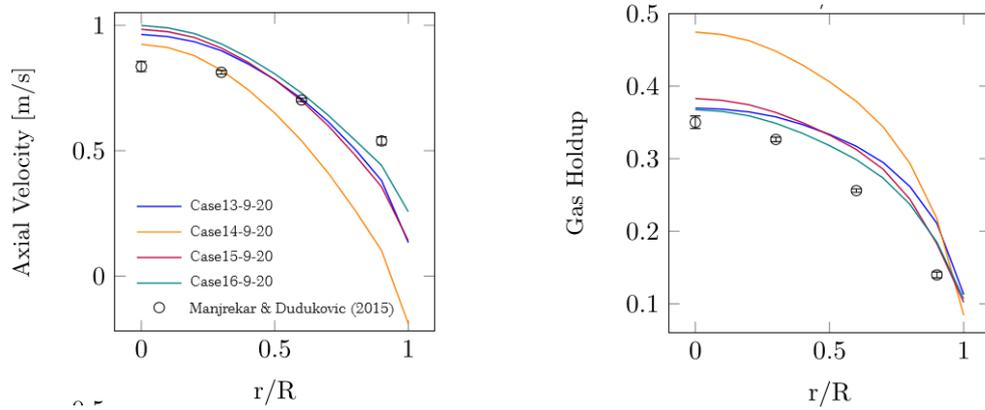
**Fig. 8.** Das (2015) coalescence model - gas superficial velocity of 20 cm/s.
