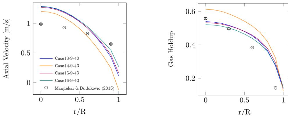
**Fig. 9.** Das (2015) coalescence model - gas superficial velocity of 40 cm/s.
