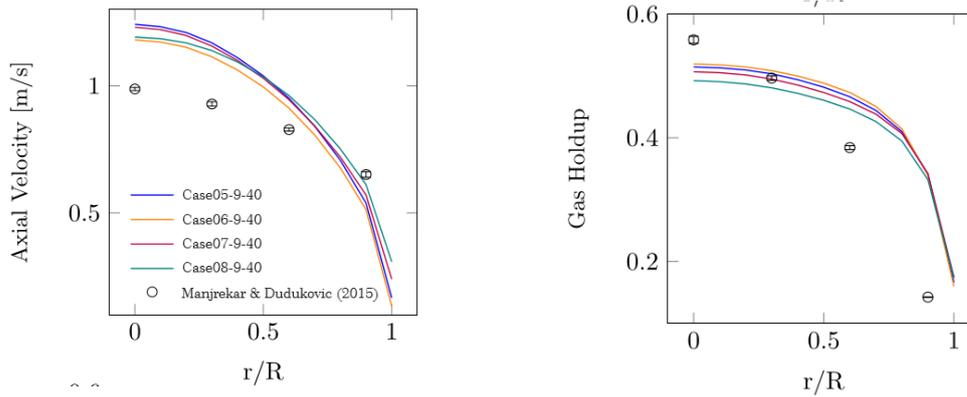
**Fig. 5. Prince and Blanch (1990) coalescence model - gas superficial velocity of 40 cm/s.**
