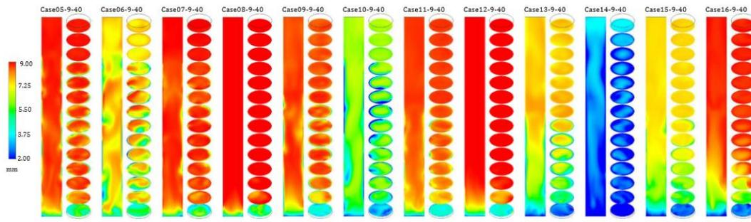
Fig. 11. Bubble size distribution - gas superficial velocity: 40 cm/s at 120 seconds.
