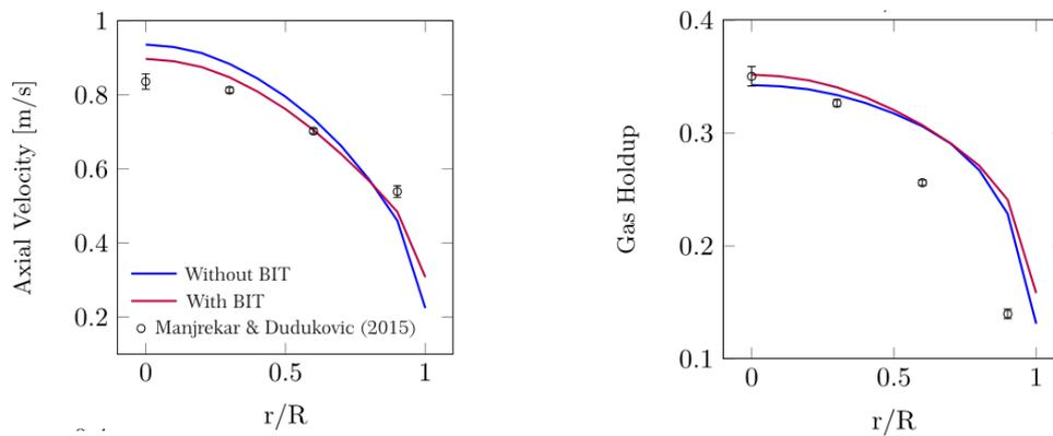
Fig. 12. Effect of bubble induced turbulence.
