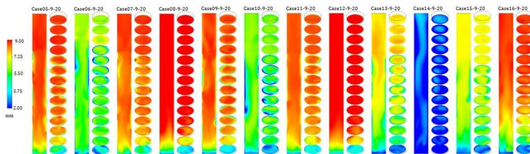
**Fig. 10.** Bubble size distribution - gas superficial velocity: 20 cm/s at 120 seconds.
