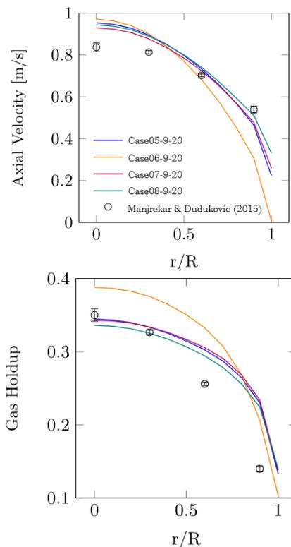
**Fig. 4. Prince and Blanch (1990) coalescence model - gas superficial velocity of 20 cm/s.**
