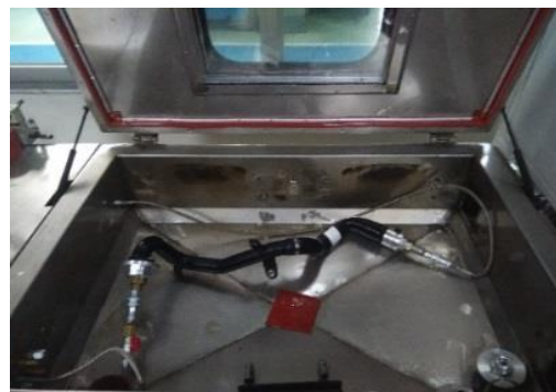
Fig. 9. Intake hose and cabined connections.
