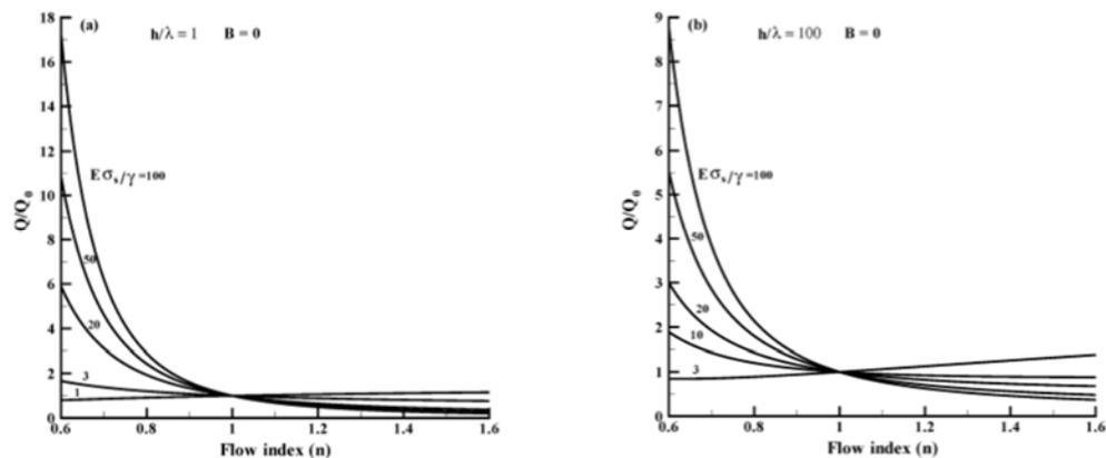
**Fig. 5.** Variation of the normalized volumetric flow rate for various salt-free power-law fluids through a cylindrical capillary without fluid slip at different values of  $E\sigma_s/\gamma$  with (a)  $h/\lambda = 1$  and (b)  $h/\lambda = 100$ . The reference flow rate  $Q_0$  is the flow rate of Newtonian fluids ( $n = 1$ ) without fluid slip ( $B = 0$ ).
