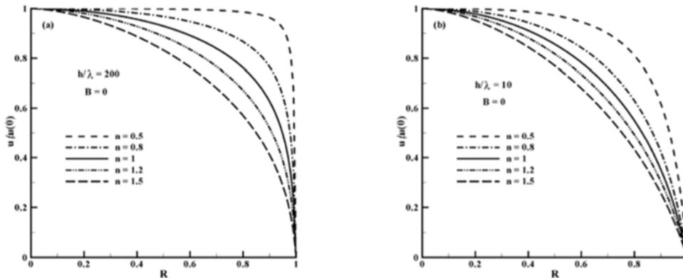
**Fig. 3.** Spatial profile of the normalized EOF velocity for various salt-free power-law fluids through a cylindrical capillary without fluid slip at (a)  $h/\lambda = 200$  and (b)  $h/\lambda = 10$ . The reference velocity  $u(0)$  is the EOF velocity at the centerline of channels.
