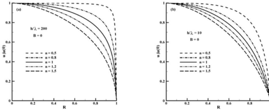
**Fig. 2.** Spatial profile of the normalized EOF velocity for various salt-free power-law fluids through a planar slit without fluid slip at (a)  $h/\lambda = 200$  and (b)  $h/\lambda = 10$ . The reference velocity  $u(0)$  is the EOF velocity at the centerline of channels.
