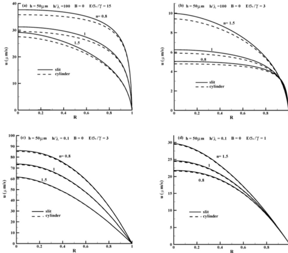
**Fig. 4.** Spatial distribution of EOF velocity for various salt-free power-law fluids through planar slit (solid lines) and cylindrical (dashed lines) micro/nanochannels without fluid slip at (a)  $h/\lambda = 100$ ,  $E\sigma_s/\gamma = 15s^{-n}$  (b)  $h/\lambda = 100$ ,  $E\sigma_s/\gamma = 3s^{-n}$  (c)  $h/\lambda = 0.1$ ,  $E\sigma_s/\gamma = 3s^{-n}$  and (d)  $h/\lambda = 0.1$ ,  $E\sigma_s/\gamma = 1s^{-n}$  with a fixed channel half-width (radius)  $h = 50\mu\text{m}$ .
