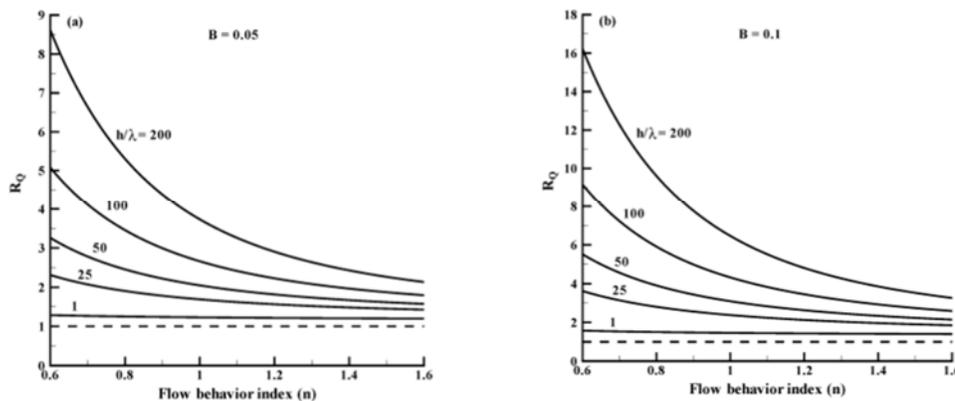
**Fig. 6.** Ratio  $R_Q$  of the flow rate with fluid slip (a)  $B = 0.05$  and (b)  $B = 0.1$  to that without fluid slip ( $B = 0$ ) in a cylindrical capillary as a function of the flow behavior index  $n$  for various values of  $h/\lambda$ . The dashed line  $R_Q = 1$  represents the case without fluid slip ( $B = 0$ ).
