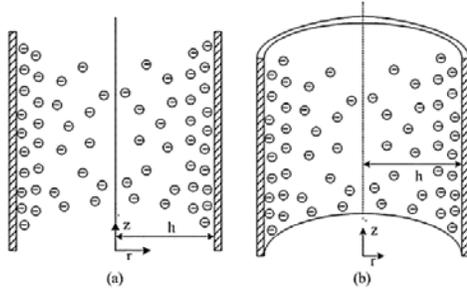
**Fig. 1. Schematic diagrams of the symmetrically charged (a) planar slit of width  $2h$  and (b) cylindrical capillary of radius  $h$ , filled with a power-law fluid containing only mobile counterions.**
