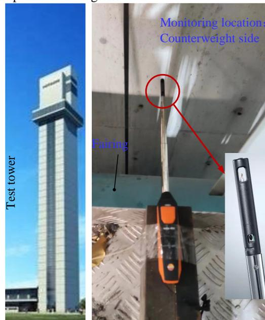
(b) Anemometer installation
