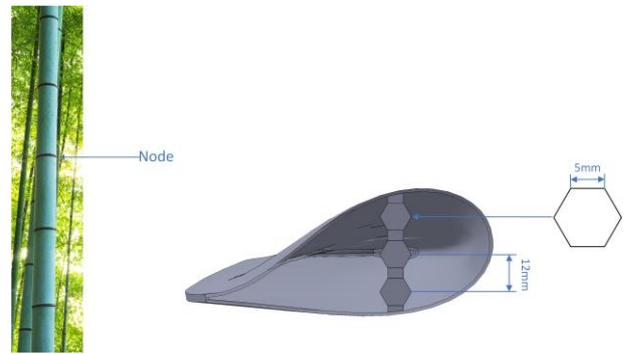
**Fig. 3** Bamboo joint distribution and bionic web
